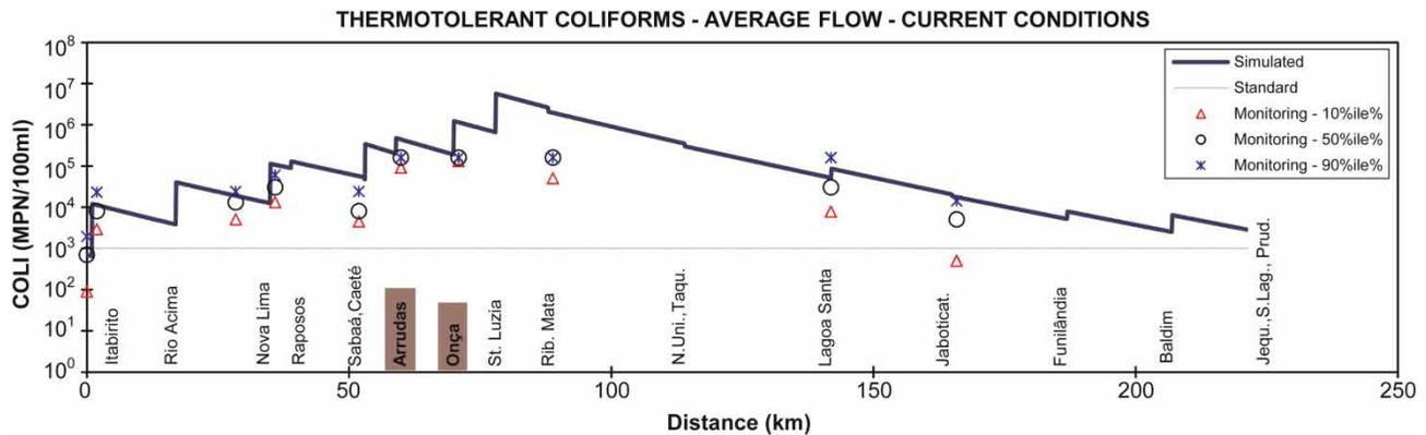
**Figure 1** | Simulation of thermotolerant coliforms in the das Velhas River. Comparison between the values simulated by the model (flow  $Q_{50}$ , current conditions) and the monitored data.
