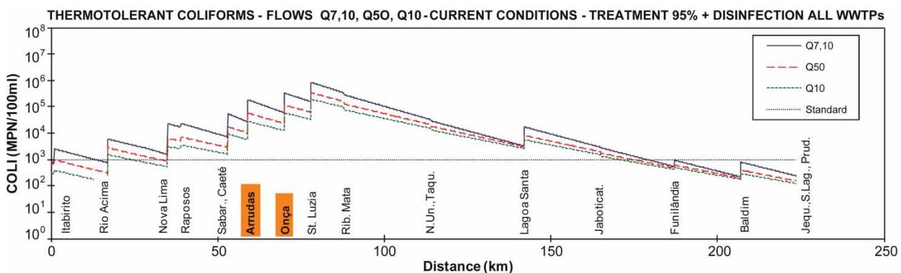
Figure 3 | Simulation of thermotolerant coliforms in das Velhas River. Current conditions. Scenario with 95% of treatment of the generated sewage and disinfection of all treated effluents in all municipalities of the study area. Flows:  $Q_{7,10}$  (dry),  $Q_{50}$  (average),  $Q_{10}$  (rainy).
