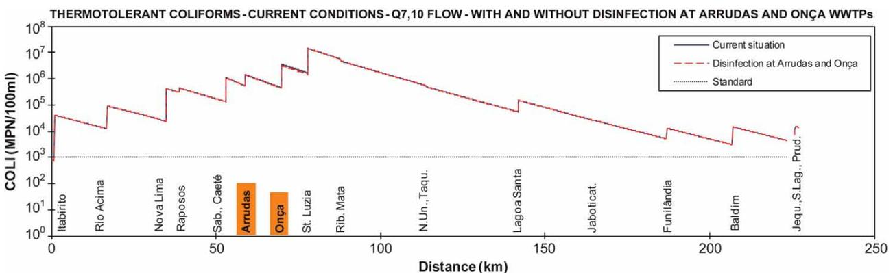
**Figure 2** | Simulation of thermotolerant coliforms in the das Velhas River. Current conditions. Flow  $Q_{7,10}$ . Scenario with and without disinfection of the effluents from the WWTPs of Arrudas and Onça.
