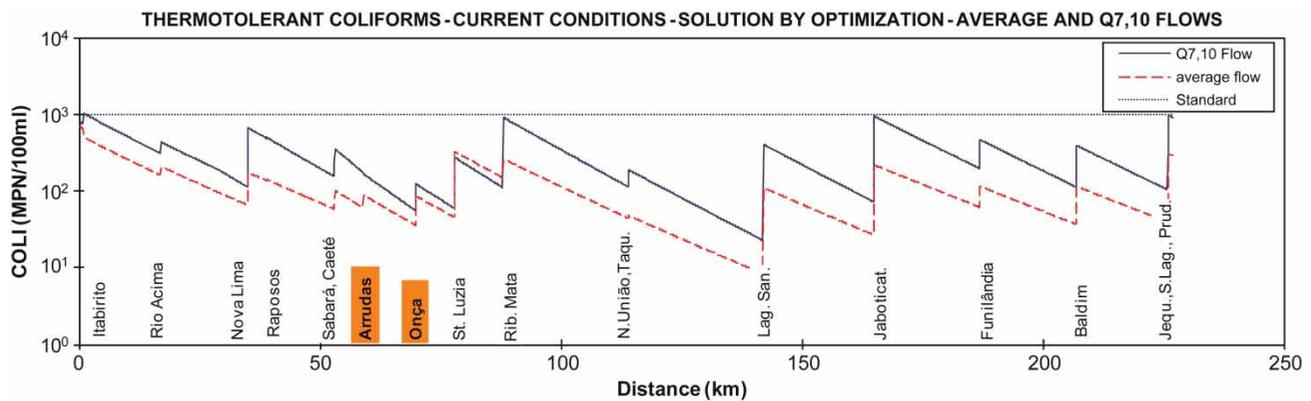
**Figure 4** | Simulation of thermotolerant coliforms in the das Velhas River. Current conditions. Scenario with the percentage of sewage treatment and coliform removal efficiency, in each municipality, defined by an optimization algorithm. Flows:  $Q_{7,10}$  and  $Q_{50}$ .
