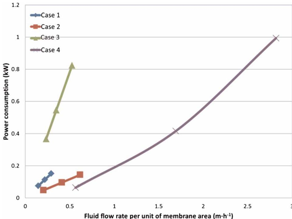
Figure 7 | Fluid flow rate per unit of membrane area vs. power consumption.
