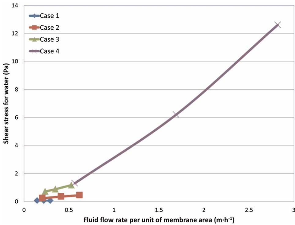
Figure 5 | Fluid flow rate per unit of membrane area vs. shear stress for water.
