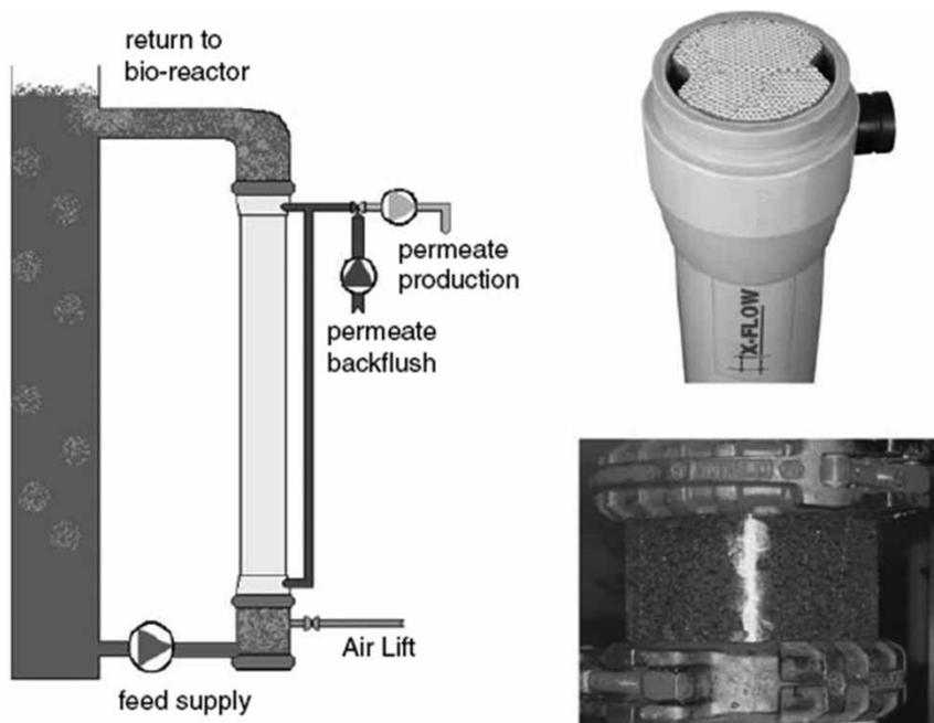
**Figure 1** | Basic principle of the Norit AirLift MBR with 8' X-Flow COMPACT membrane module and continuous aeration (Futselaar *et al.* 2007).
