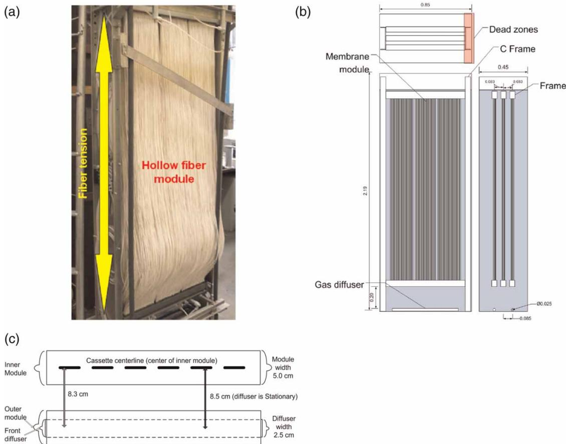
**Figure 2** | (a) Cassette frame with membrane modules, (b) membrane module and diffuser location in MBR pilot plant, and (c) location of the diffusers with respect to the membrane modules (Fulton 2009).
