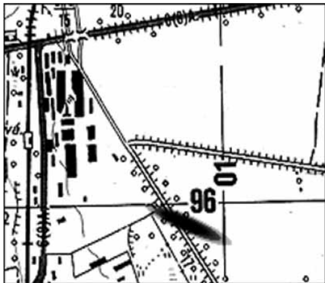
Figure 4 | Estimated soil water pollution at aluminium smeltery, Apc, 150 days after the break down.
