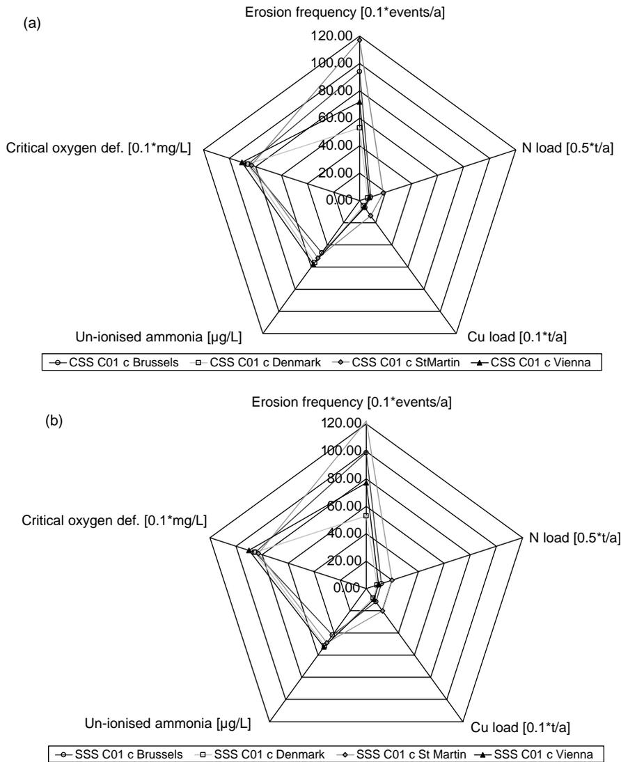
**Figure 2** Different types of rain: alpine (St Martin), continental (Vienna) and oceanic (Brussels, Copenhagen), performance of (a) combined system (CSS) and (b) separate system (SSS) in catchment 1 (100 ha, 70 PE/ha) with high pollution (concentration c). Note that each axis has a different scaling
