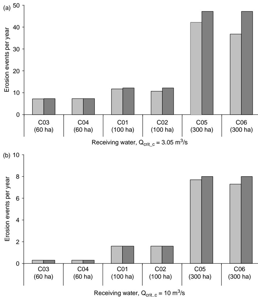
**Figure 4** Number of erosion events per year: catchments C1, C2, C3, C4, C5 and C6, erosion frequency in a small receiving water RW with  $Q_{crit,c}$   $3.05 \text{ m}^3/\text{s}$  (left) and a larger RW with  $Q_{crit,c}$   $10 \text{ m}^3/\text{s}$  (right). Alpine rain (St Martin). The lighter colour represents the combined, the darker one the separate system
