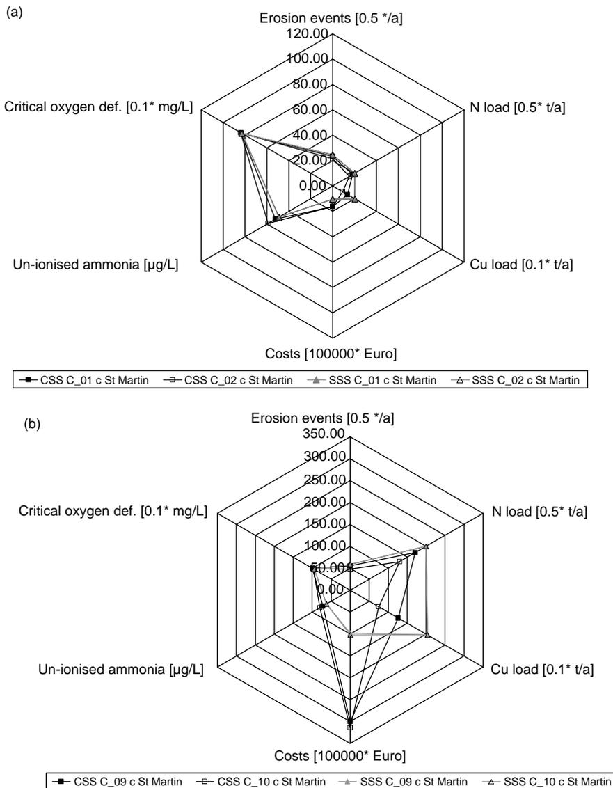
**Figure 1** Combined and separate system impacts calculated for a catchment of 100 ha (a) with 70 PE/ha (C1) 200 PE/ha (C2) and of 1,000 ha (b) with 70 PE/ha (C9) 200 PE/ha (C10), respectively. High pollution (concentration c), alpine rain (St Martin, Austria). Note that each axis has a different scaling
