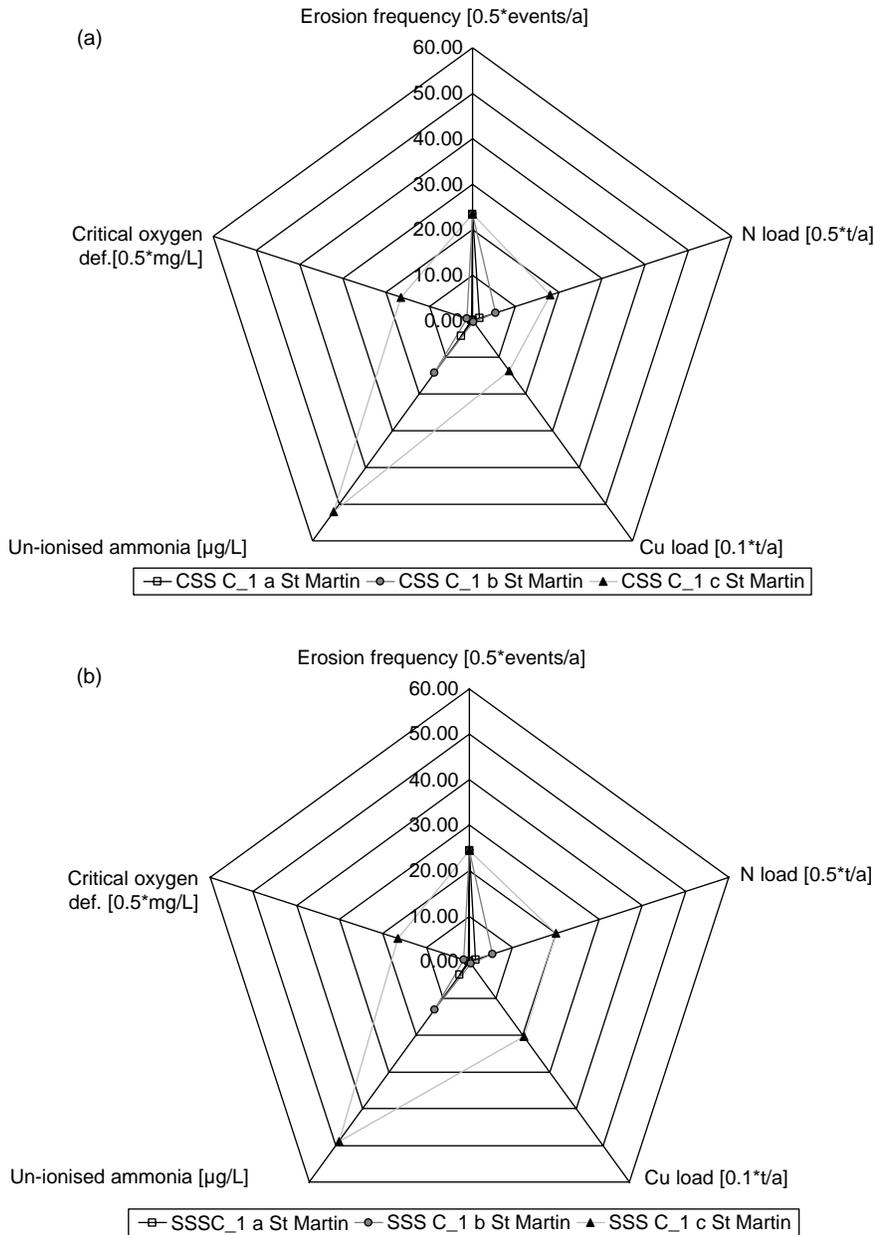
**Figure 3** Different pollution concentrations (a- low, b- median, c- high) in stormwater and dry weather flow, performance of combined system (CSS) and separate system (SSS) in catchment 1 (100 ha, 70 PE/ha) calculated with alpine rain (St Martin). Note that each axis has a different scaling
