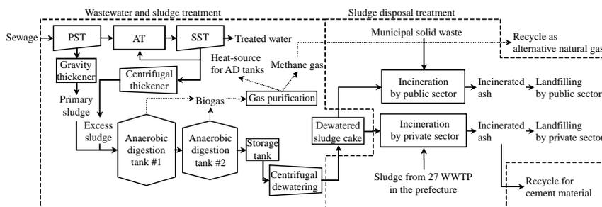
Figure 2 The current flow-scheme of sludge treatments for the city
