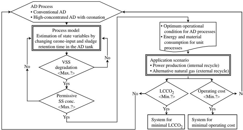
**Figure 4** The algorithm seeking the optimum process scheme
