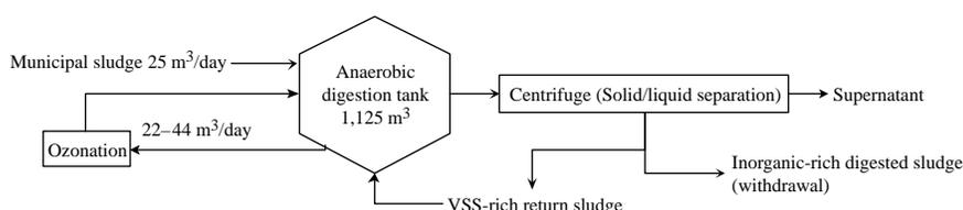
**Figure 1** Process scheme of the test reactor – the high-concentrated anaerobic digestion with partial ozonation of digested sludge
