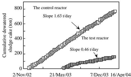
**Figure 7** The production of dewatered sludge cake
