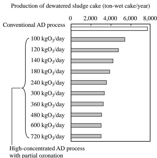
**Figure 9** Expected dewatered sludge cake production
