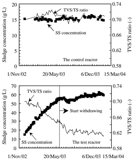
**Figure 5** The trend of SS concentration and TVS/TS ratio (top: the control reactor, bottom: the test reactor)
