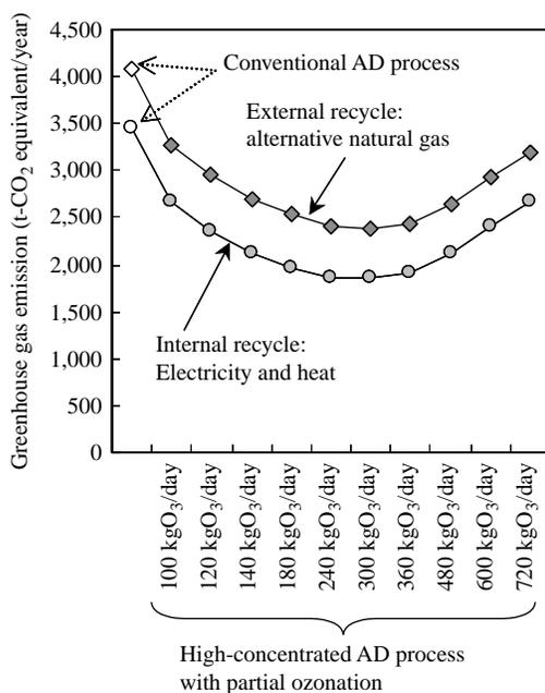
**Figure 10** The estimation of greenhouse gas emission in sludge treatment and disposal in the city
