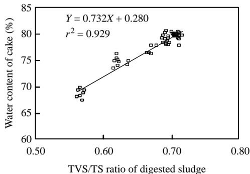
**Figure 8** Reduction of cake volume by lowering TVS/TS ratio of sludge
