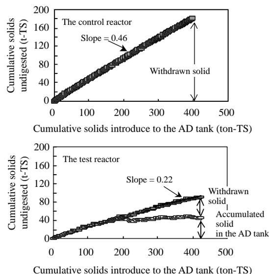
**Figure 6** The fraction of undigested sludge (top: the control reactor, bottom: the test reactor)
