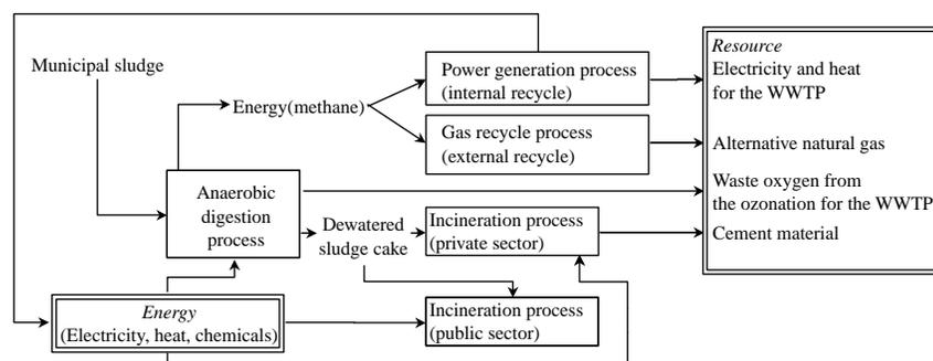
**Figure 3** The energy and material-flow matrix of the city for municipal sludge treatments and disposal processes
