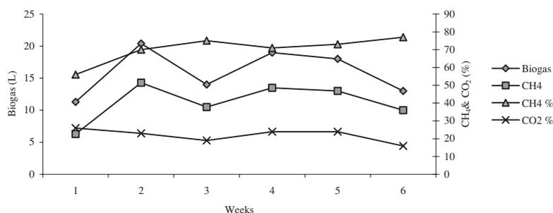
**Figure 4** Biogas production in degradation of grass in two stage anaerobic reactor
