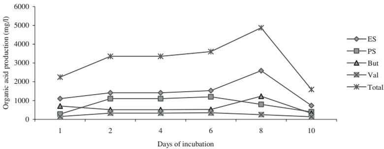
**Figure 2** Production of organic acids from the reactor inoculated with cattle dung slurry
