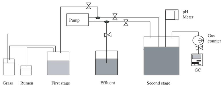
**Figure 1** Small scale two stage anaerobic digester used for degradation of grass
