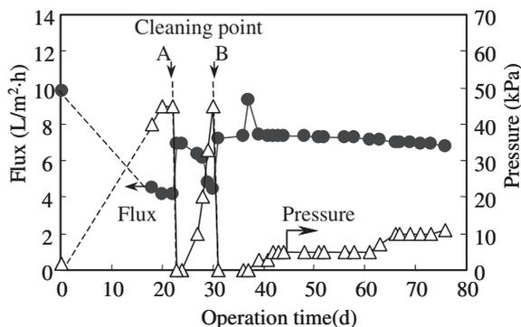
**Figure 1** Variations of flux and transmembrane pressure in the intermittently aerated SMBR during the operation time
