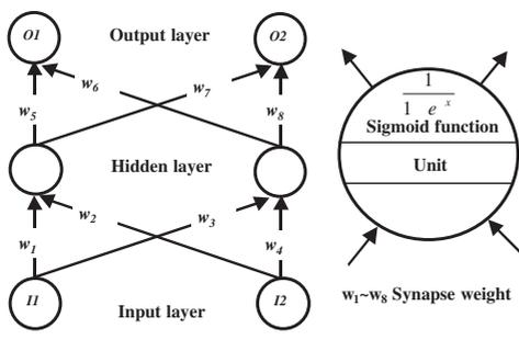
**Figure 2** A three-layered artificial neural network and transfer function in unit
