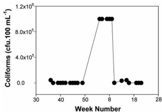
**Figure 5** | Estimation of faecal coliforms in treated water from the IAPS at point of discharge. Composite samples were harvested weekly over a 24 h period for 8 months. Data are the mean of three independent determinations.
