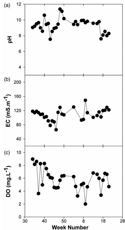
**Figure 2** | Physicochemical characteristics of water following sewage treatment using an IAPS. (a) pH, (b) EC, and (c) dissolved oxygen (DO) were determined for composite samples collected weekly for 24 h over a period of 8 months. Data presented are the average of duplicate measurements.
