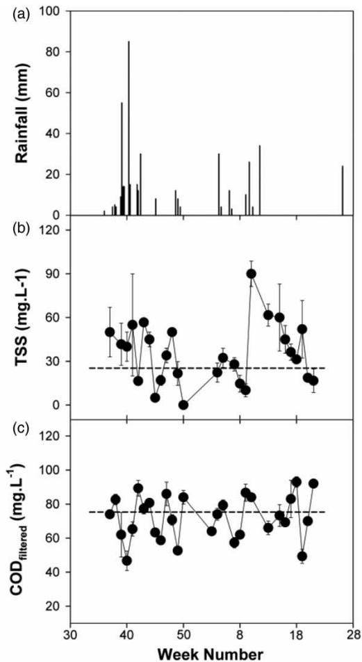
**Figure 3** | Relationship between rainfall events and TSS and COD of treated water from the IAPS at point of discharge. (a) Precipitation was recorded weekly and, (b) TSS and (c) COD ( $\text{COD}_{\text{filtered}}$ ) were determined for composite samples harvested weekly over a 24 h period for 8 months. Stippled line indicates the General Limit Values for TSS and  $\text{COD}_{\text{filtered}}$ . Data presented are the average of duplicate measurements.
