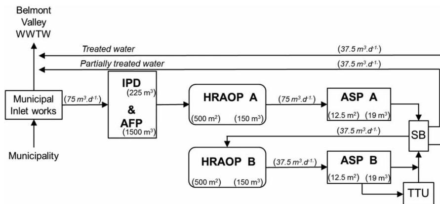
**Figure 1** | Process flow and configuration of the experimental IAPS located at the Belmont Valley WWTW. The system receives raw sewage, screened for the removal of plastics via a grit and detritus channel. Pond and reactor surface area, volume, and flow rates are shown in parentheses. Effluent enters at the bottom of the IPD some 6 m below water level. SB = splitter box; TTU = tertiary treatment unit.
