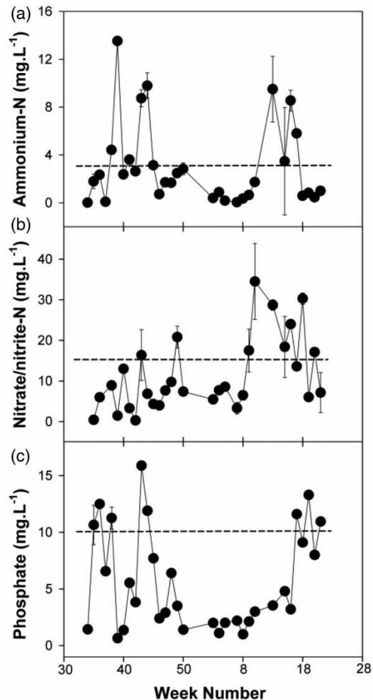
**Figure 4** | Nutrient content and composition of treated water from the IAPS at point of discharge. (a) Phosphate, (b) nitrate/nitrite-N and (c) ammonium-N concentrations in composite samples harvested weekly over a 24 h period for 8 months were determined using test kits as described in the 'Materials and methods' section. Stippled line indicates the General Limit Values for each parameter. Data presented are the average of duplicate measurements.
