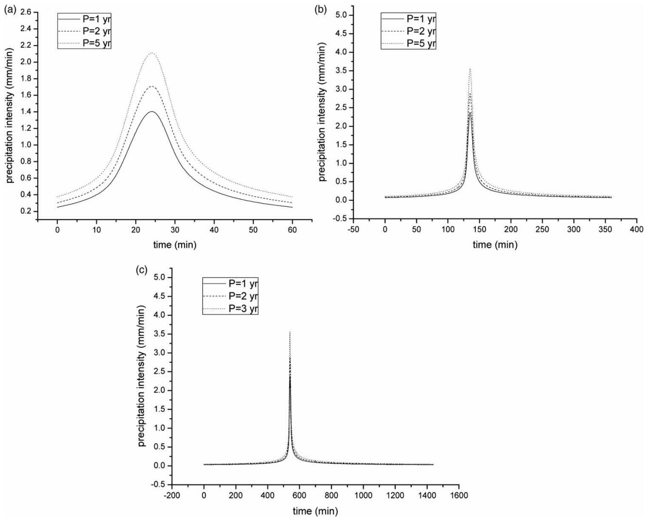
**Figure 3** | IDF curves (a) rainfall duration = 60 min, (b) rainfall duration = 360 min, (c) rainfall duration = 1,440 min.
