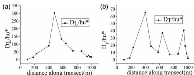
Figure 7 | Transverse variation of dimensionless dispersion coefficients  $D/hu^*$ .
