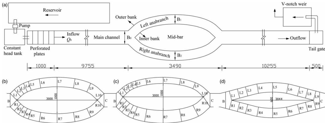
**Figure 1** | Diagram of the experimental model (a), and location diagrams of measured sections with (b) case 1 with  $B^* = 0.5$ , (c) case 3 with  $B^* = 0.33$  and (d) case 4 with  $B^* = 0.5$  (length unit: mm).
