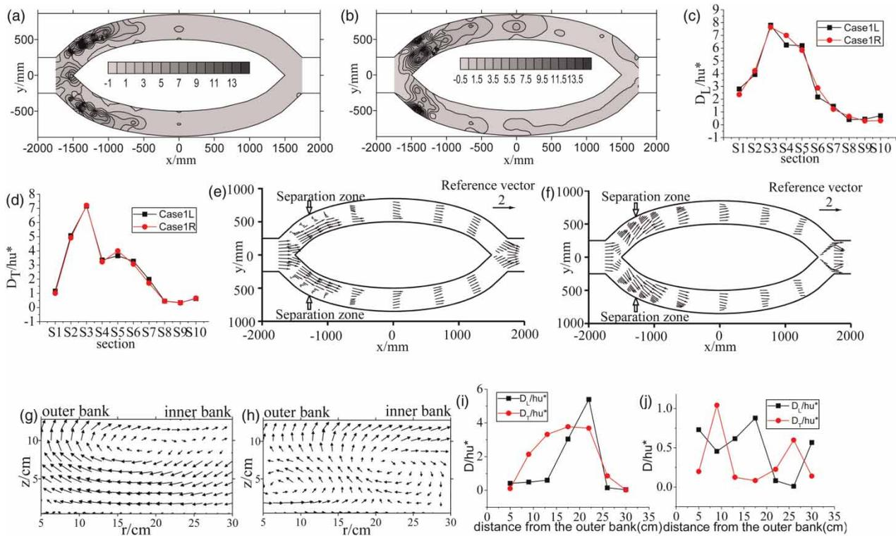
**Figure 2** | Distributions of  $D_L/hu^*$  and  $D_T/hu^*$  and the flow structure in case 1: (a) contour of  $D_L/hu^*$ , (b) contour of  $D_T/hu^*$ , (c) section-averaged  $D_L/hu^*$ , (d) section-averaged  $D_T/hu^*$ , (e) flow field at the surface ( $z = 12.7$  cm), (f) flow field at the bottom ( $z = 0.5$  cm), (g) and (h) secondary flow in L7 and L9, (i) and (j) transverse variation in L7 and L9.
