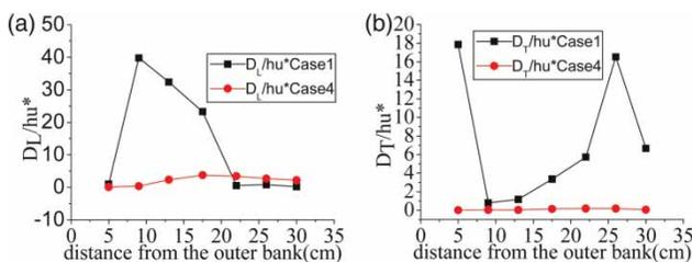
Figure 5 | Transverse variation of  $D/hu^*$  in section L3 for cases 4 and 1: (a)  $D_L/hu^*$ , (b)  $D_T/hu^*$ .
