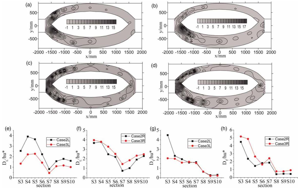
**Figure 3** |  $D_L/hu^*$  and  $D_T/hu^*$  in cases 2 and 3: (a) and (b) contour of  $D_L/hu^*$  in case 2 and 3, (c) and (d) contour of  $D_T/hu^*$  in cases 2 and 3, (e) and (f) section-averaged  $D_L/hu^*$  of the left and right anabranch, (g) and (h) section-averaged  $D_T/hu^*$  of the left and right anabranch.
