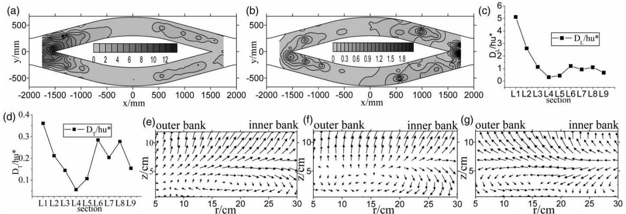
**Figure 4** |  $D_L/hu^*$  and  $D_T/hu^*$  and flow structure in case 4: (a) contour of  $D_L/hu^*$ , (b) contour of  $D_T/hu^*$ , (c) longitudinal variation of section-averaged  $D_L/hu^*$ , (d) longitudinal variation of section-averaged  $D_T/hu^*$ , (e)–(g) secondary current in L2, L4, and L7.
