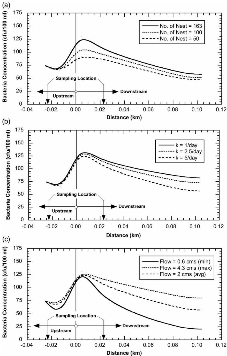
**Figure 3** | Effect of (a) number of bridge-dwelling birds, (b) decay rate and (c) channel flow on *E. coli* concentration in downstream.
