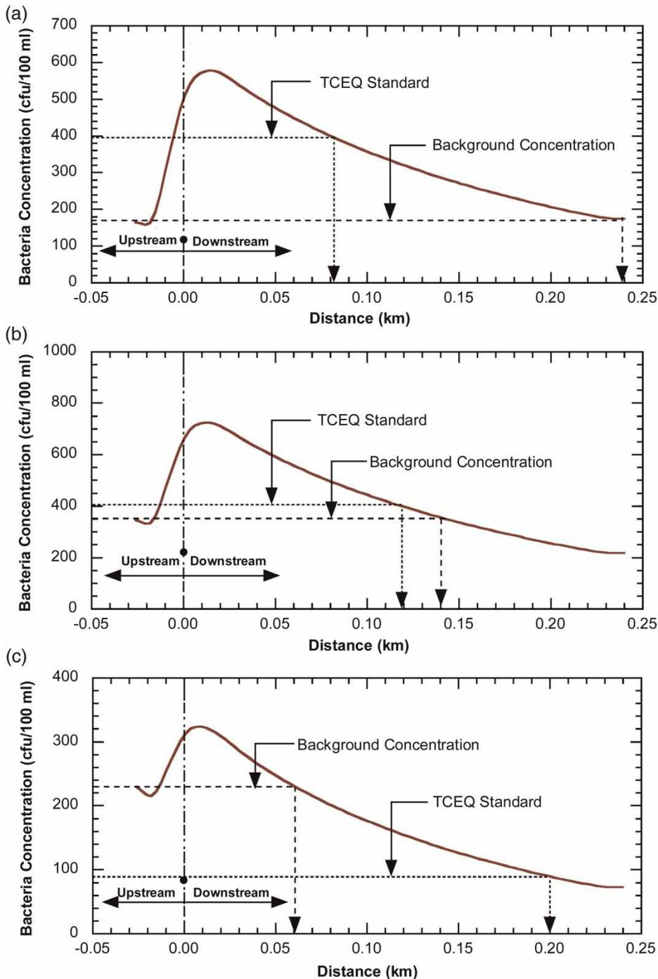
Figure 5 | Predicted Impaired Sections: (a) *E. coli*, (b) fecal coliform and (c) enterococci.
