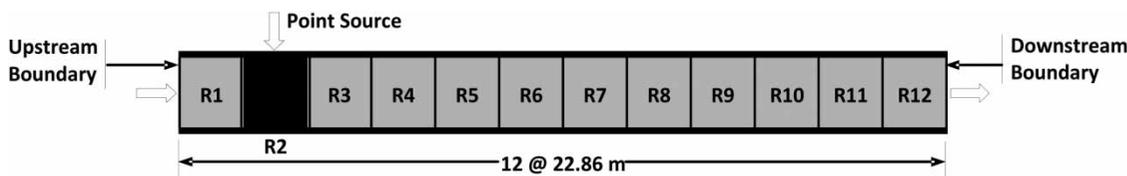
**Figure 2** | QUAL2Kw segmentation scheme.
