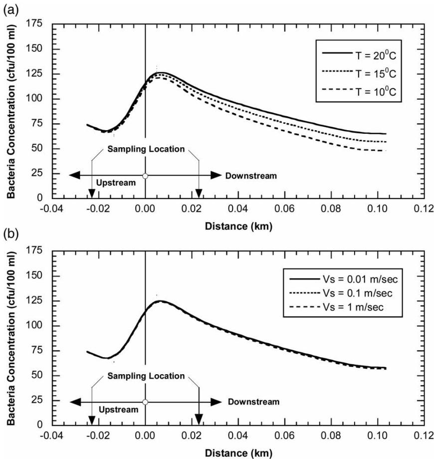
**Figure 4** | Effect of (a) water temperature and (b) settling velocity on *E. coli* concentration.
