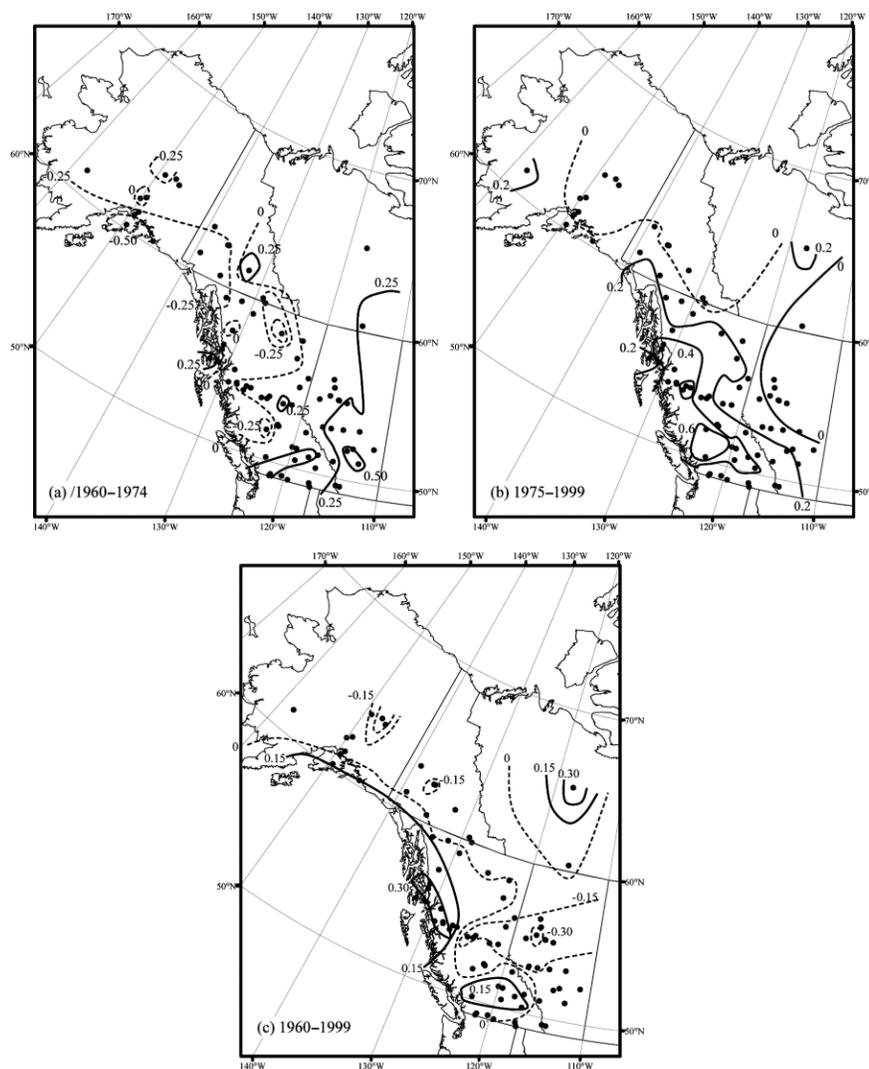
**Figure 5** | Trends in mean streamflow (discharge correlated against time) for 1960–1999, 1960–1974 and 1975–1999 periods for the spring season (April–June). Solid or dashed isolines of  $r$  values indicate positive or negative correlation, respectively. Trend is statistically significant at 5% where  $|r| \geq 0.3$  for the 1960–1999 series; where  $|r| \geq 0.5$  for the 1960–1974 series; and where  $|r| \geq 0.4$  for the 1975–1999 series.
