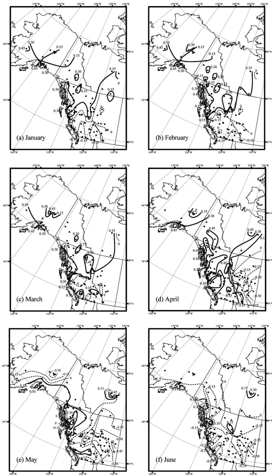
**Figure 3** | Spatial patterns of correlation ( $r$  values) between mean flows of January–June (a)–(f), and October–March PDO. Dots indicate location of stations that provide data for this study. Solid or dashed isolines indicate positive or negative correlation, respectively. Correlation is significant at 5% where  $|r| \geq 0.30$ .
