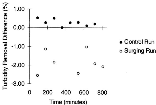
Fig. 5 Effect of surges on turbidity removal.
