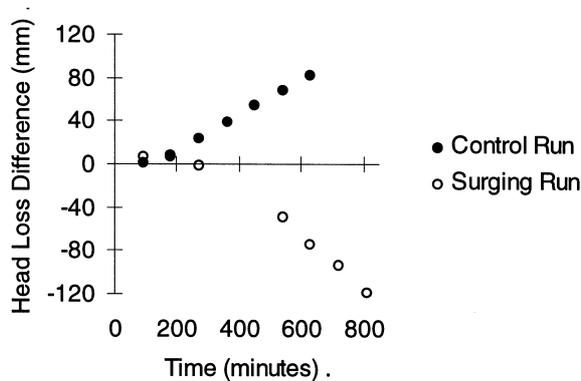
Fig. 4 Effect of surges on head loss development.
