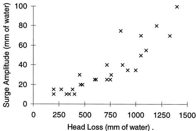
Fig. 2 Pressure fluctuations in the filtrate piping at plant B.
