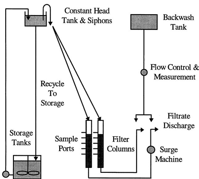
Fig. 3 Experimental apparatus used to investigate surging.
