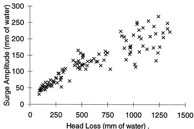
Fig. 1 Pressure fluctuations in the filtrate piping at plant A.
