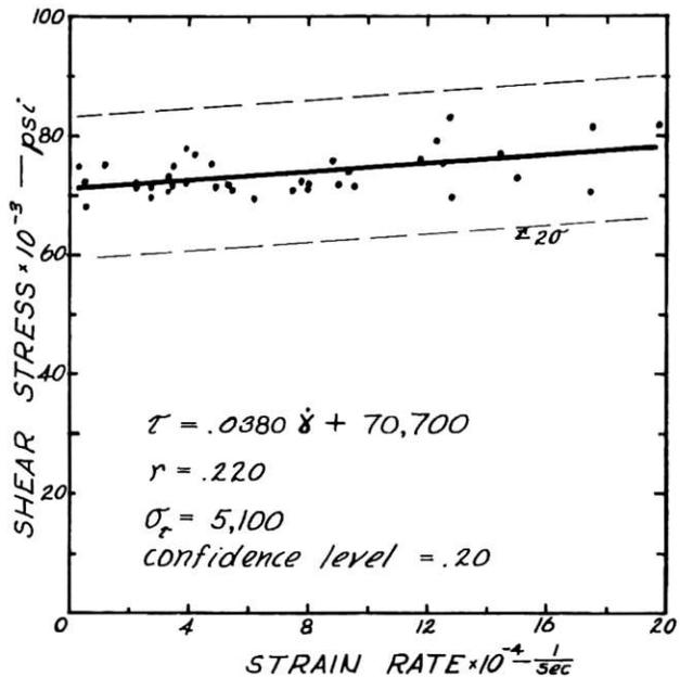
Fig. 12 Variation of shear stress with strain rate (from Kececioglu)
