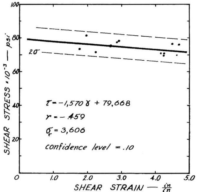
Fig. 11 Variation of shear stress with strain (from Kececioglu)
