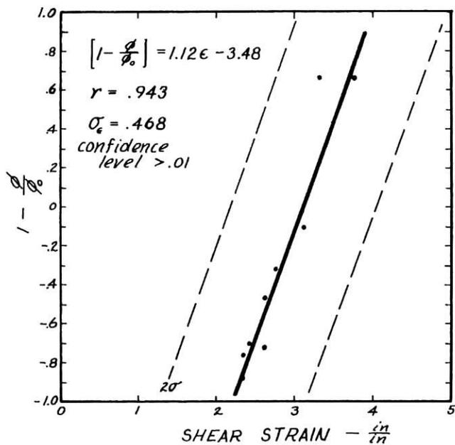
Fig. 13 Data from Bagley and Mennell; C-6 carbide cutting 235 Bhn, 4340 steel; tool signature of 0, 0, 5, 5, 5, 0, 0.020; 0.200 depth, 0.005 feed; dry; V = 50 to 700 sfpm
