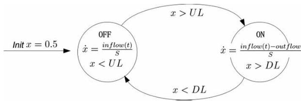
Figure 1 | Pump station autonomous hybrid automaton.
