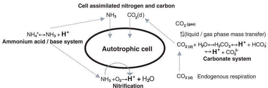
**Figure 1** Schematic of dynamic processes that effect system pH
