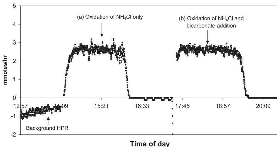
**Figure 4** Measured HPR for nitrification. (a) addition of  $\text{NH}_4\text{Cl}$  only, (b) addition of  $\text{NH}_4\text{Cl}$  and bicarbonate
