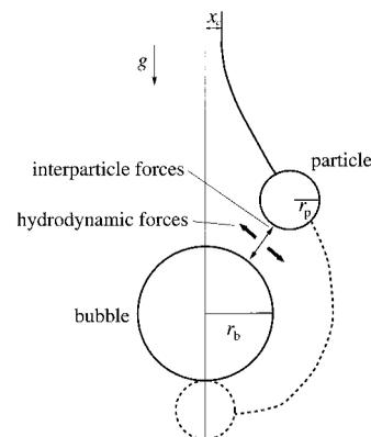
**Figure 1** | The approach of a rising bubble and a falling particle indicating the influence of hydrodynamic forces and interparticle forces. The dashed line is the continuation of the particle trajectory indicating particle capture at the rear of the bubble.
