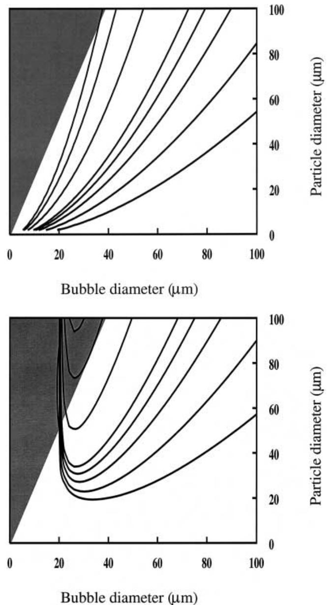
**Figure 3** | Contour plots of flotation rate constant  $R$  for particles with  $\zeta_p = -40$  mV (a) and  $\zeta_p = 0$  mV (b). From the bottom right inwards the contour values are  $R = 0.1, 0.25, 0.5, 0.75, 1.0, 2.5, 5.0,$  and  $7.5$   $\text{s}^{-1}$ .
