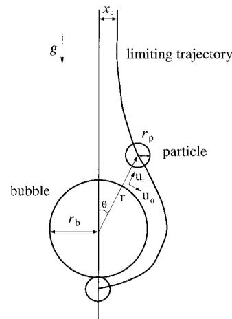
Figure 2 | Coordinate system used to model relative particle trajectories around the bubble.
