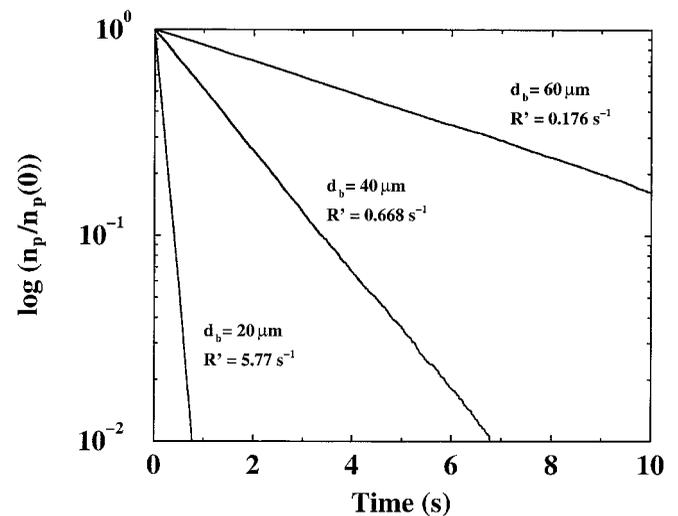
**Figure 5** | Particle log fractions as a function of time for particles of size  $d_p = 30 \mu\text{m}$  using bubbles of size  $d_b = 20 \mu\text{m}$ ,  $d_b = 40 \mu\text{m}$  and  $d_b = 60 \mu\text{m}$ .
