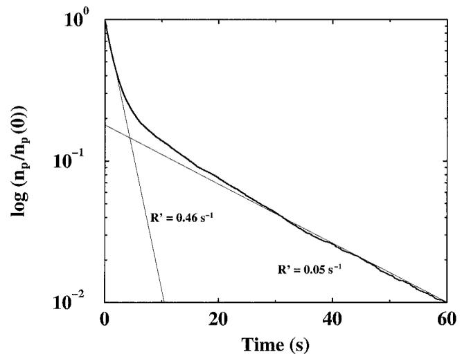
Figure 7 | Particle log fraction as a function of time for the bimodal particle distribution given in Figure 6 showing the asymptotic flotation rates at short and long times.
