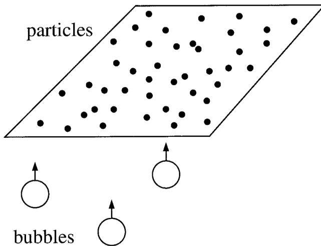
**Figure 4** | Schematic of the random arrangement of particles and injection of bubbles used in the statistical model.
