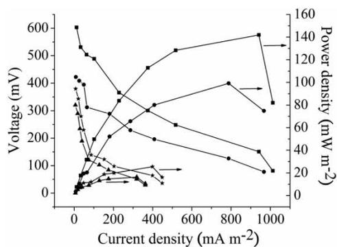
**Figure 3** | Polarization and power density curves of MFCs operating on 1,000  $\text{mg L}^{-1}$  glucose (■) and 1,000  $\text{mg L}^{-1}$  glucose containing different concentrations of metronidazole (10  $\text{mg L}^{-1}$  ●, 30  $\text{mg L}^{-1}$  ★, 50  $\text{mg L}^{-1}$  ▲) at an external resistance of 1,000  $\Omega$ . The arrows indicate the corresponding curves were the power density curves.
