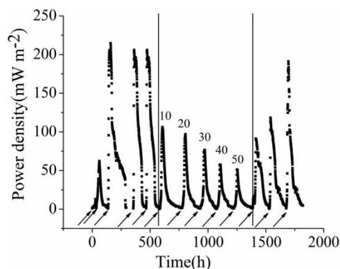
**Figure 1** | Power production from MFCs in the presence of glucose, and glucose with metronidazole (arrows indicate when reactors were fed with fresh medium; numbers indicate the concentration of metronidazole ( $\text{mg L}^{-1}$ )) under external resistance of 1,000  $\Omega$ .
