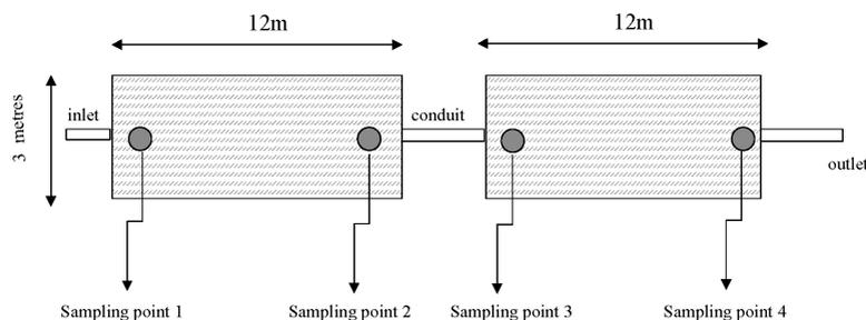
**Figure 1** Schematic diagram of wetland together with biofilm sampling sites
