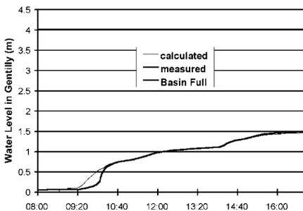
**Figure 5** Hydraulic calibration during wet weather (29/10/96 rainfall): Gentilly basin
