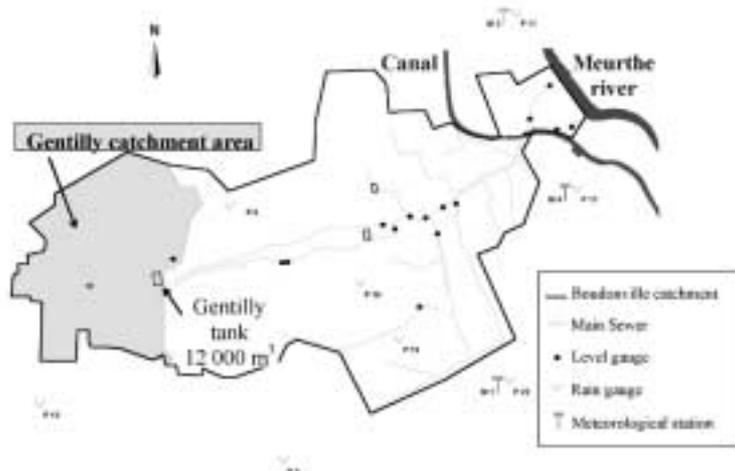
**Figure 1** General description of the site and the measurement points
