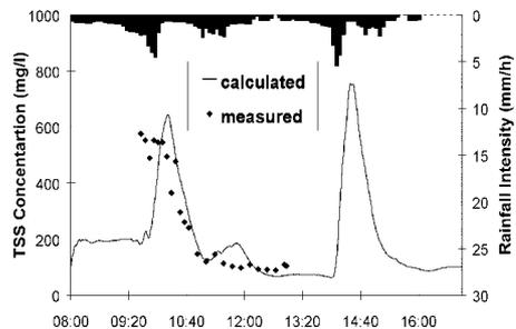
**Figure 6** Pollution calibration during wet weather (29/10/96 rainfall): Jacquinet point
