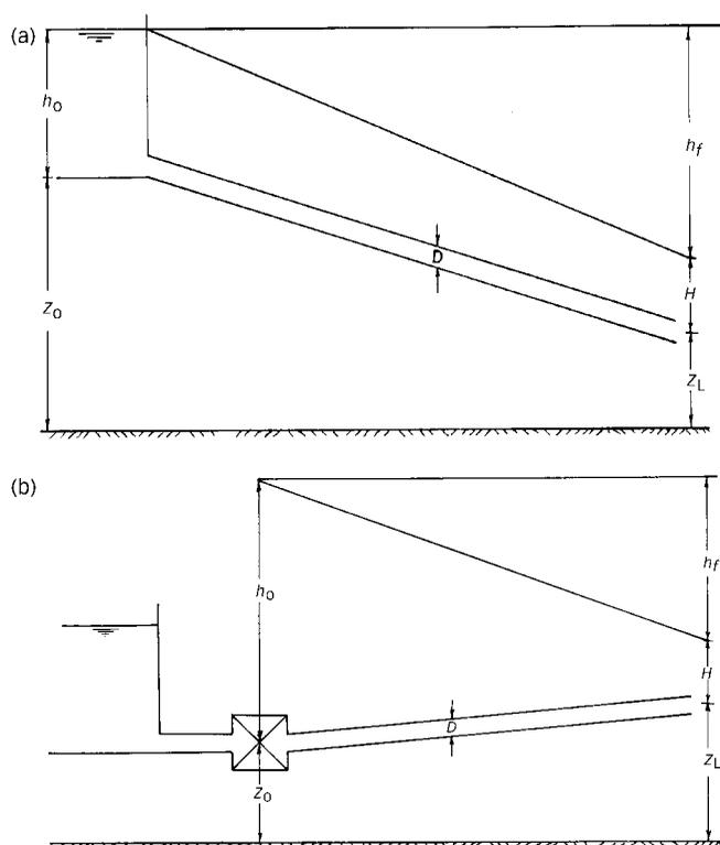
Figure 1 | Definition sketch: (a) gravity main; (b) pumping main.
