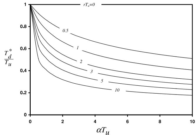
Figure 2 | Variation of design period of a gravity main.
