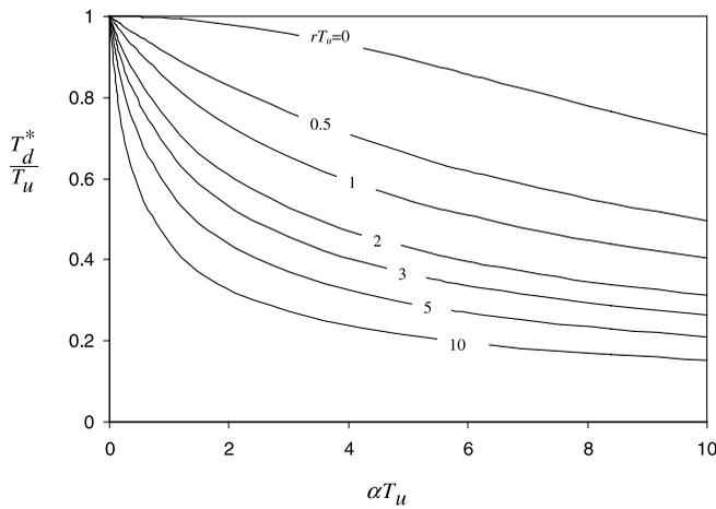
Figure 3 | Variation of design period of a pumping main.
