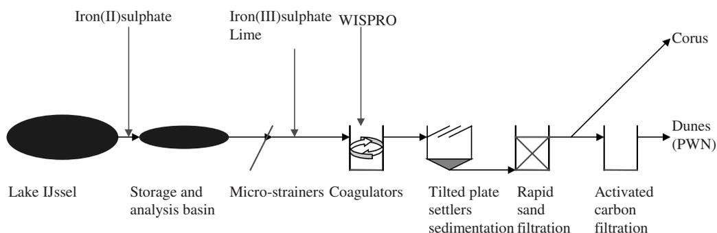
**Figure 1** | A schematic representation of the processes in the water treatment plant 'Prinses Juliana' at Andijk.
