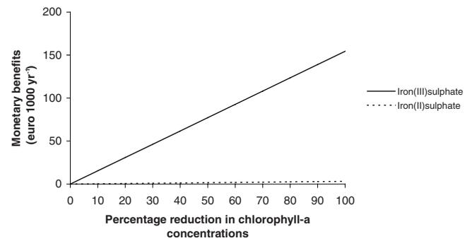
**Figure 8** | Cost savings for the water treatment plant at Andijk when iron(II)sulphate and when iron(III)sulphate are used as steering variables, depending on reductions in chlorophyll-a concentrations in Lake IJssel compared with the situation in 1985.
