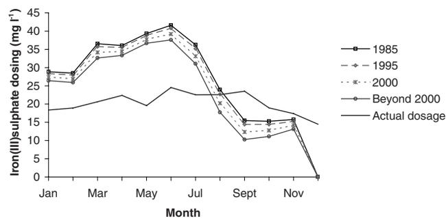
**Figure 7** | Iron(III)sulphate dosage in the coagulation process for different scenarios and actual dosage for 1995.
