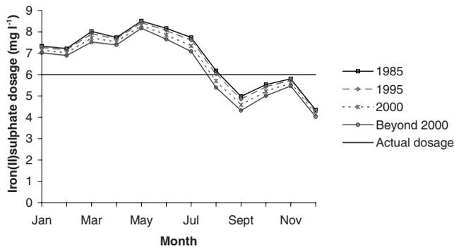
**Figure 6** | Iron(II)sulphate dosage in the basin for different scenarios and actual dosage for 1995.
