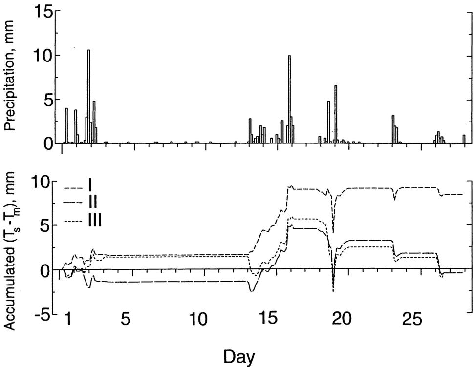
Fig. 4. Three-hour total precipitation and accumulated difference between simulated throughfall ( $T_s$ ) and measured throughfall ( $T_m$ ) for November 1990. Simulations were made using three different parameter sets (I-III).
