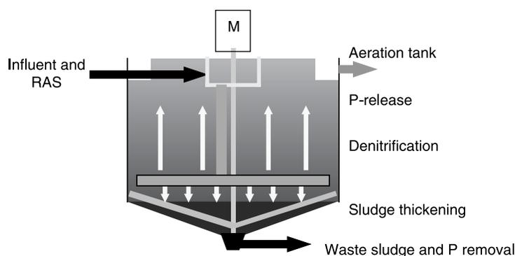
**Figure 1** Schematic diagram of UMBR
