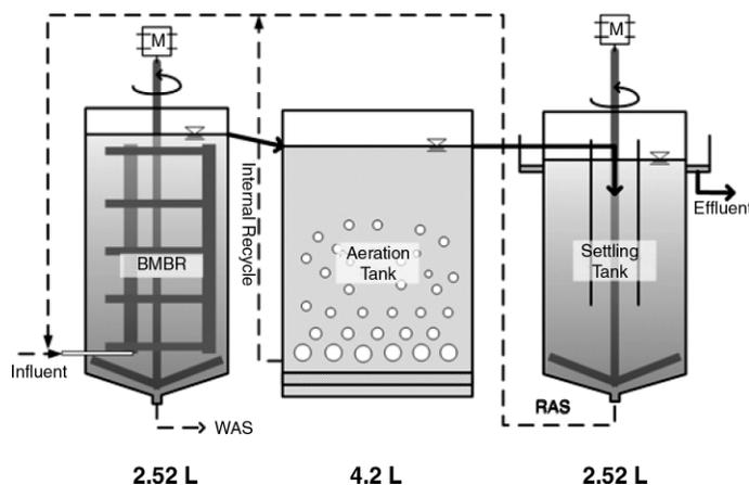
**Figure 2** Schematic diagram of laboratory scale KNR<sup>®</sup> process
