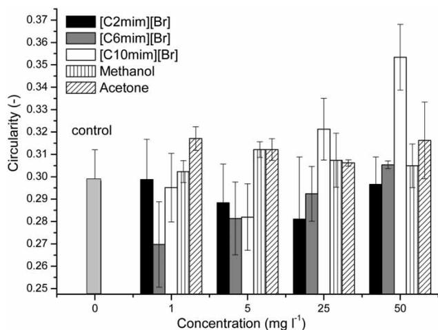
**Figure 2** | Comparison of the mean circularity of activated sludge flocs exposed to the tested ILs or traditional organic solvents and not exposed to these chemicals after 24 hours of testing.
