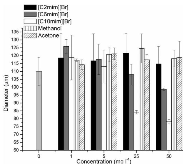
Figure 1 | Comparison of the mean diameter of activated sludge flocs exposed and not exposed to ILs or traditional solvents after 24 hours of testing.
