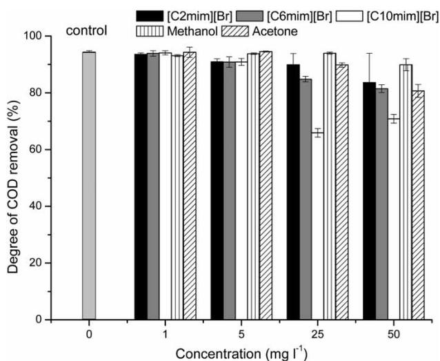
**Figure 4** | Comparison of the degree of COD removal after 24 hours of testing.
