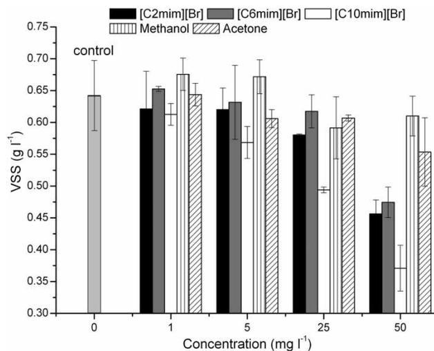
**Figure 3** | Comparison of biomass concentration in the experiments with ionic liquids and traditional organic solvents added to wastewater after 24 hours of testing.
