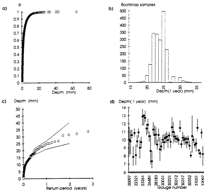
Fig. 2. The estimation procedure. (a) The empirical distribution function at gauge 30031 for depth. (b) The histogram for depth (1 year) estimated by means of the bootstrap resampling method used on the observed rain events. (c) The return periods and the estimated 90% control confidence intervals. (d) The estimated 90% central confidence intervals for all 56 gauges for depth (0.1 year).
