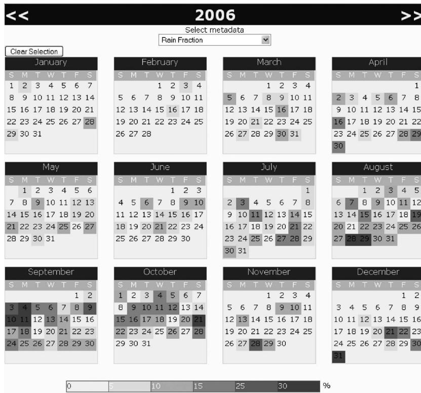
Figure 2 | Calendar view of Hydro-NEXRAD metadata. Darker color indicates higher metadata value. This visual inspection tool can help identify days with significant precipitation events.
