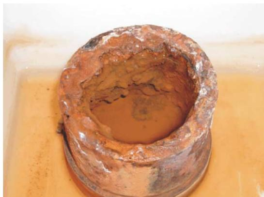
**Figure 1** | Photograph of 4 inch diameter cast-iron pipe section used in study.
