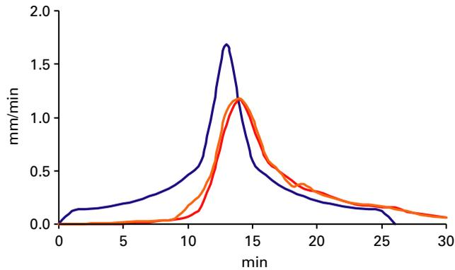
**Figure 3** Runoff from 2 m long experimental green roof study plot with drainage layer sloping 3% and 20% (almost identical lower curves) as a result of artificial Lund design rain (upper curve). Excess storage 4 mm
