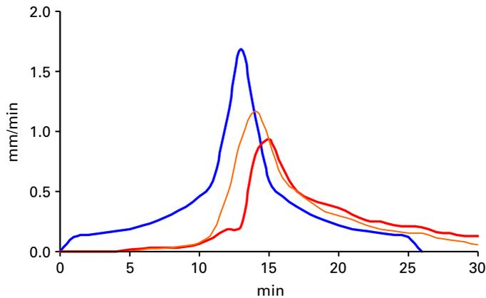
**Figure 5** Runoff from 2 m long experimental roof plot sloping 7% with drainage layer (thin middle curve) and without drainage layer (lowest curve) generated by artificial design rain (uppermost symmetrical curve)
