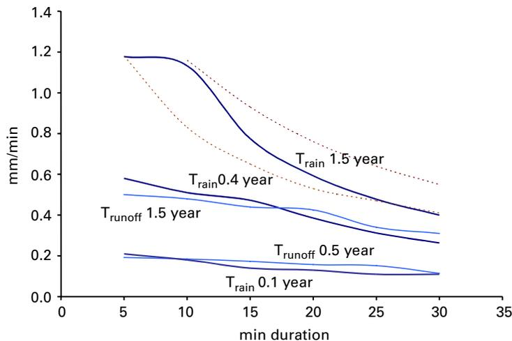
**Figure 6** Intensity–duration–frequency curves ( $T_p$  for rain and  $T_q$  for runoff with return period in years as index) from 3 cm sedum-moss roof in Augustenborg, Malmö. Maximum rain and runoff represent 1.5 year return period. The dashed lines shows intensity–duration curves with return period 1.5 and 3 year as given by Niemczynowicz (1982)
