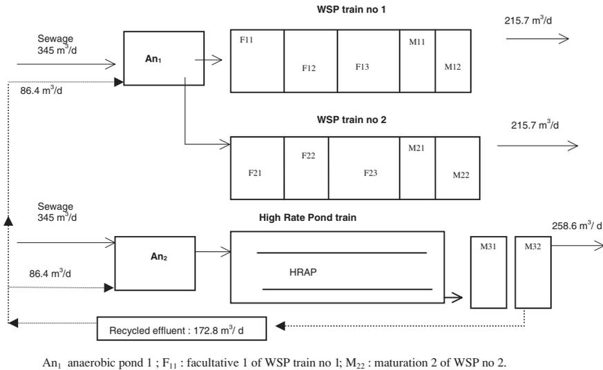
**Figure 1** Layout of experimental wastewater treatment facilities at Ouarzazate (Morocco)
