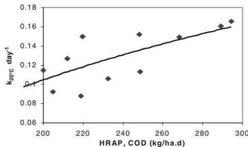
**Figure 2** Linear regression analysis between the COD loading rate and COD removal,  $k_{20^\circ\text{C}}$  in the HRAP (Ouarzazate, Morocco)
