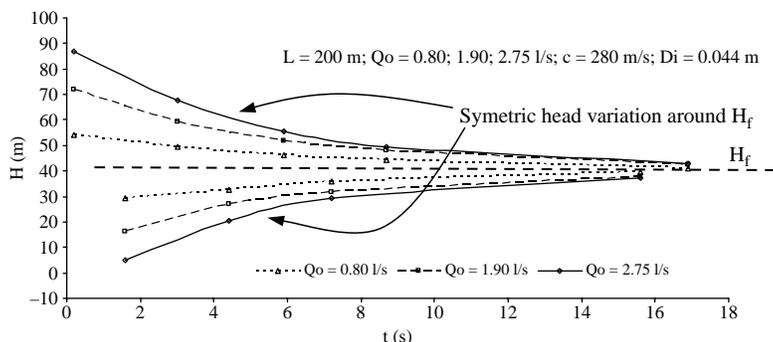
Figure 7 | Effect in a plastic pipe due to viscoelasticity and friction.
