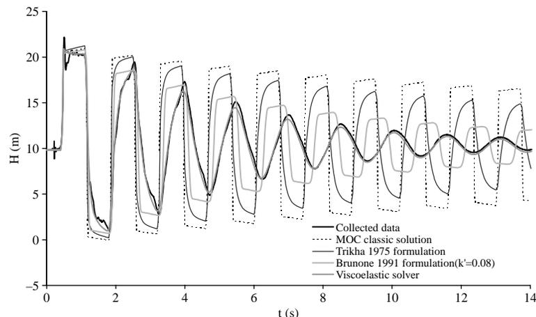
Figure 13 | Piezometric head at the downstream end of experimental facility 2: transient data vs numerical simulations.
