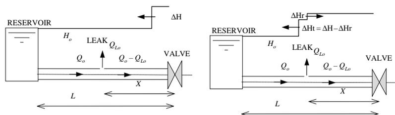
Figure 15 | Topology of the system. Pressure surge generated by a leak.
