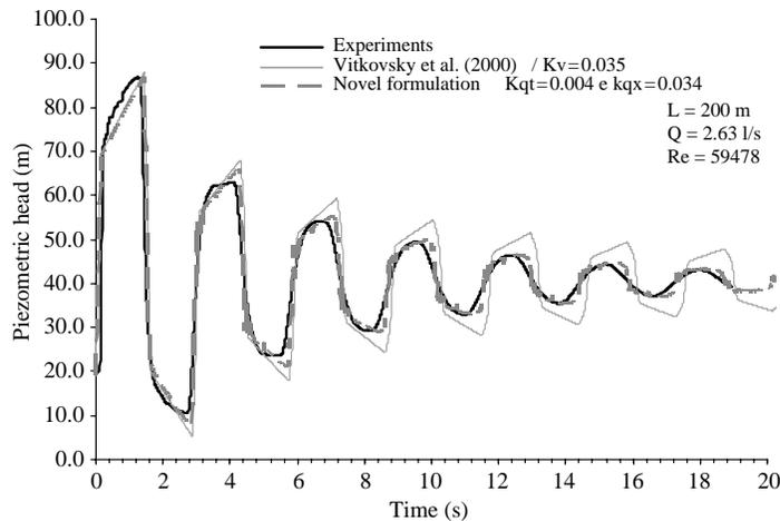
**Figure 9** | Comparisons between experiments and transient roughness models.
