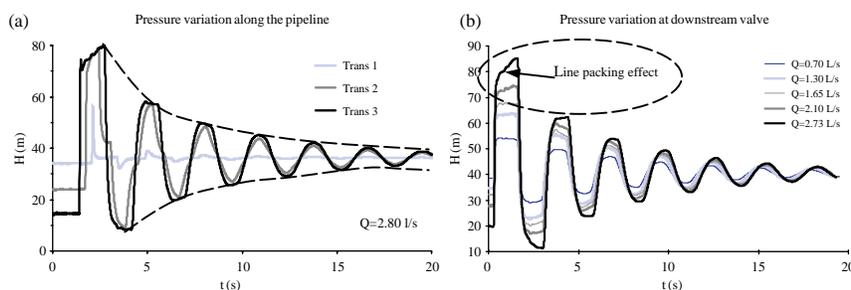
**Figure 6** | Experimental tests in facility 1: a) pressure variation along the pipe (for different positions of transducers); b) pressure variation at the valve for different discharge values.
