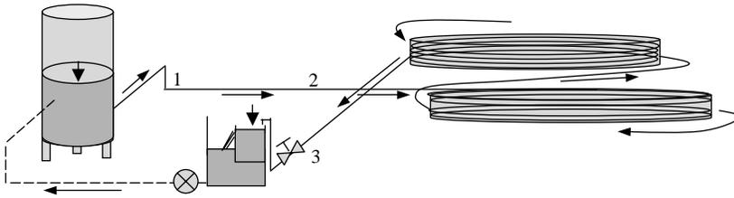
**Figure 1** | Scheme of experimental facility 1 with HDPE pipe ( $L = 200$  m).
