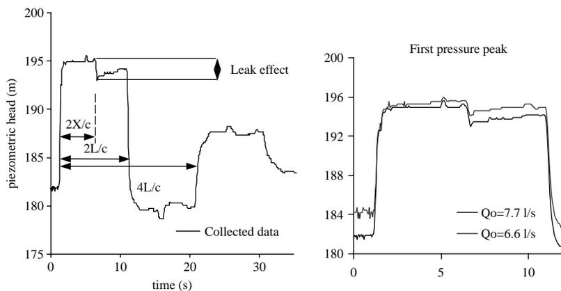
**Figure 17** | Lintrathen East Trunk Main Network (Balmashanner). Leak effect in the piezometric head variation due to a fast downstream valve closure.
