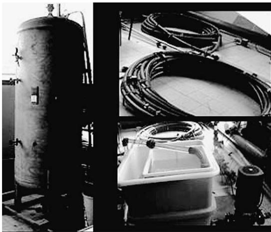
**Figure 2** | Details of experimental facility 1: pressurised tank, coils of HDPE pipe and downstream tank.
