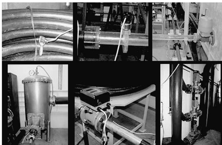
**Figure 4** | Details of experimental facility 2 (from left to the right, top to the bottom): pipe coil, pressure transducer, diaphragm valve, air vessel, flow meter and pumps.
