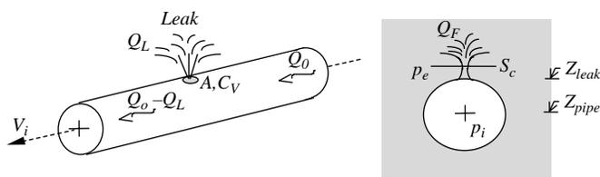
Figure 14 | Schematic presentation of a leak. Physical fundamental parameters.
