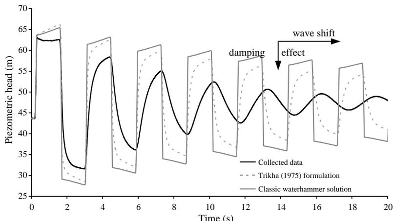
Figure 8 | Effect and wave dispersion in a plastic pipe due to viscoelasticity and friction influence.
