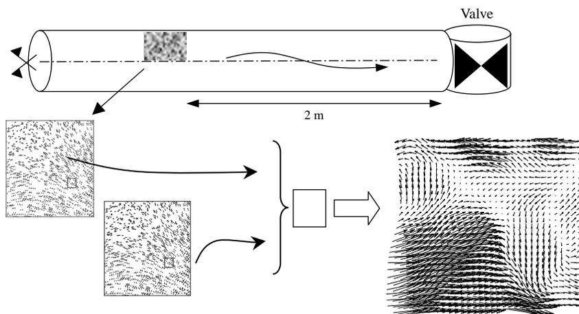
**Figure 10** | Application of the PIV technique in a perspex pipe of experimental facility 2 for field velocities achievement (Hacamo 2002).
