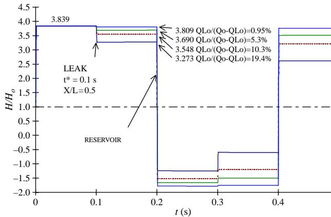
**Figure 16** | Pressure surge generated by an instantaneous total valve closure in a simple hydraulic system with a leak at the middle of the pipeline obtained by MOC.
