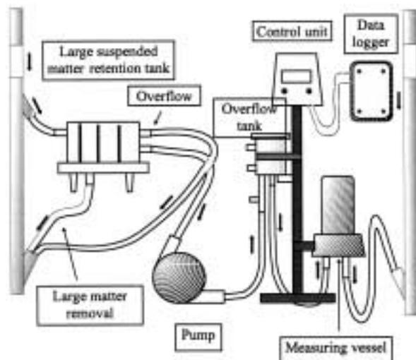
**Figure 2** Feeding system and optical device
