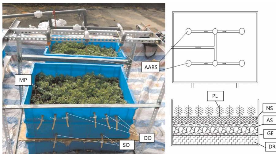
**Figure 1** | Green roof trays on the rooftop in Tianjin University, China (MP: *Sedum lineare* Thunb.; AARS: adjustable artificial rainfall sprinklers; OO: overflow outlet; SO: sampling orifice; PL: plant layer; NS: nutrient substrate; AS: adsorption substrate; GE: geotextile; and DR: drainage system).
