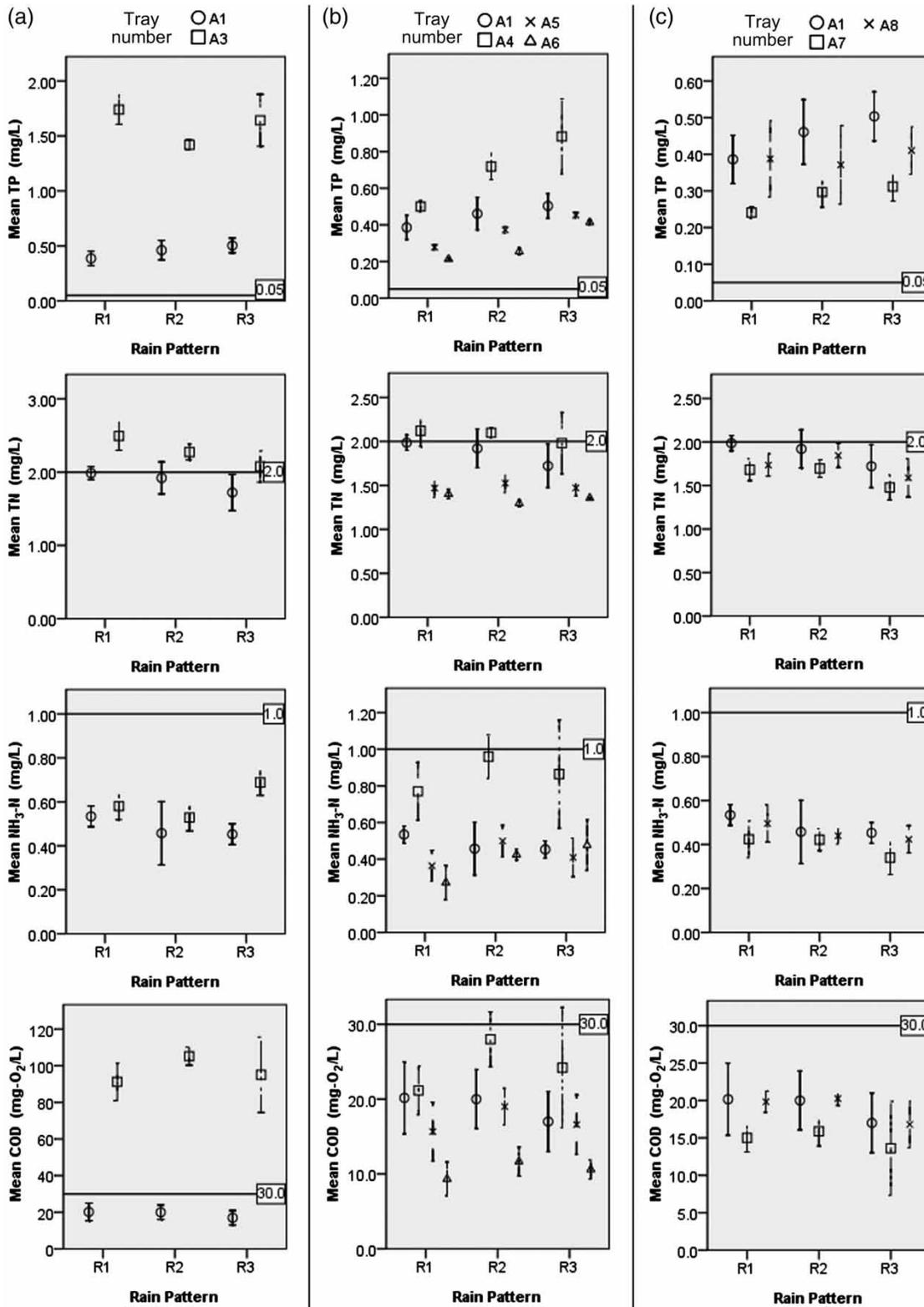
**Figure 2** | Nutrient pollutant concentrations in the runoff at different artificial rain events from different trays. (As the type of extensive green roof that tray A1 represented is the most commonly used in China and its unit cost per area is relatively low, A1 was selected as the benchmark for other trays.)
