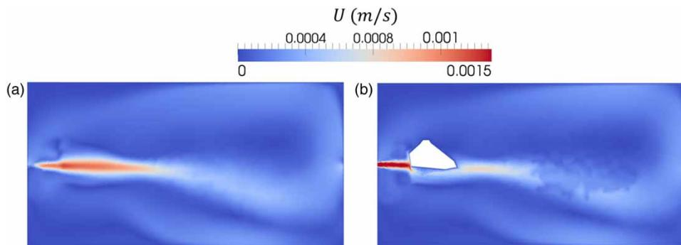
**Figure 2** | Flow velocity contours based on 3D CFD model (a) at 0.1 m and (b) at 0.7 m below the water surface (1.7 m and 1.1 m above the bottom of the pond, respectively). Note: the blank portion near the inlet at 0.7 m below the water surface represents the extent of accumulated sludge at that level.
