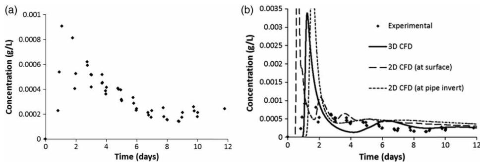
**Figure 1** | Results of (a) the dye tracer field study, superimposed with (b) the results from the CFD simulations.
