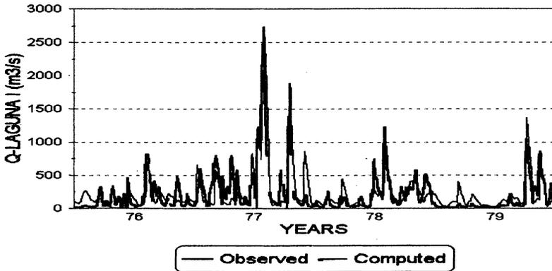
Fig. 4. Calibration: Daily observed and computed runoff.
