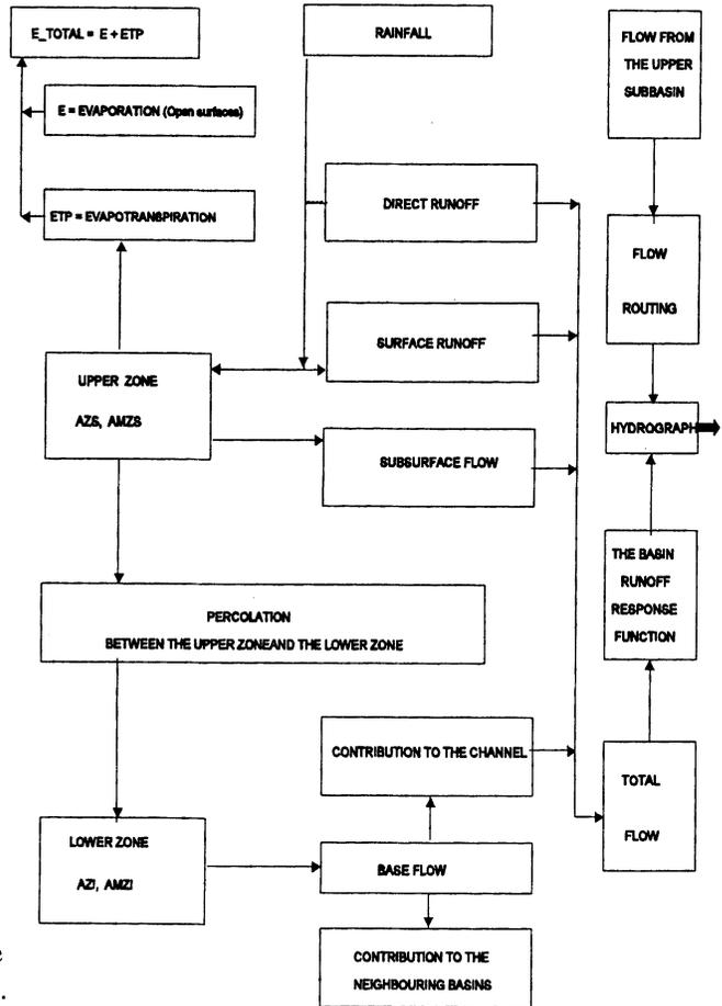
Fig. 2. Flow diagram of the Hydro-Urfing model.
