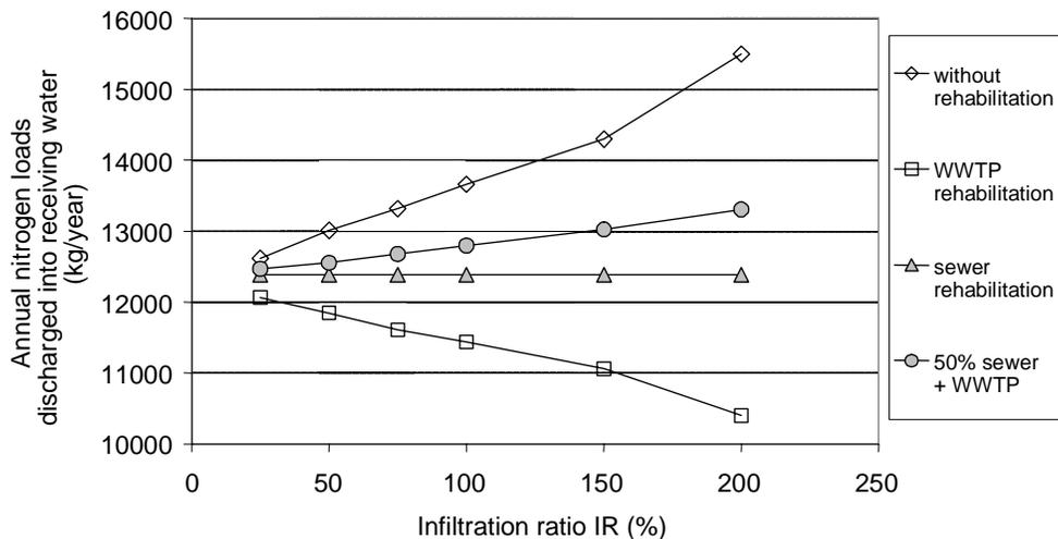
Figure 3. Annual NGL loads discharged into the receiving water vs. IR and strategy.
