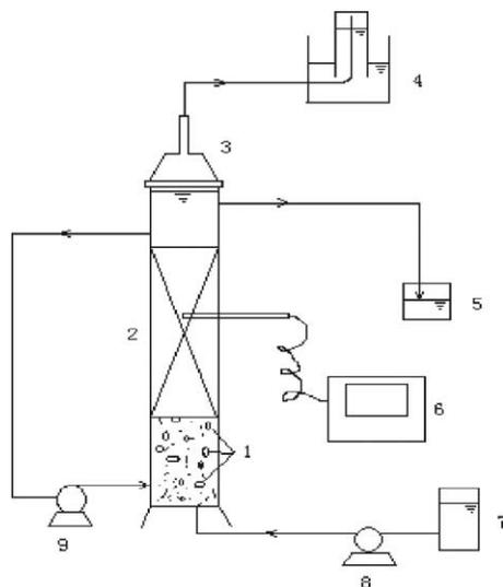
**Figure 1** Schematic of anaerobic attached-growth bioreactor. 1 Suspended-growth zone; 2 Attached-growth zone; 3 Gas collection zone; 4 Gas collection apparatus; 5 Effluent zone; 6 Temperature controller; 7 Influent zone; 8 Influent pump; 9 Recirculating pump
