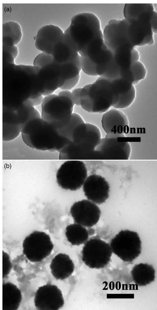
**Figure 1** | TEM images of the prepared  $\text{Fe}_3\text{O}_4$  (a) and  $\text{Fe}_3\text{O}_4/\text{CS}$  (b).
