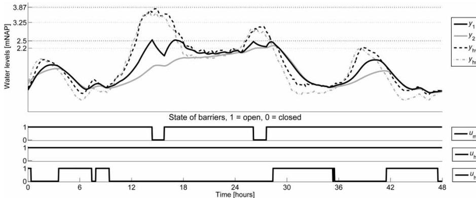
**Figure 15** | Simulation results of the TIO-MPC approach for scenario 1. The dotted horizontal lines represent respectively from bottom to top the reference levels  $r_{21}$ ,  $r_{11}$ ,  $r_{22}$  and  $r_{12}$ .
