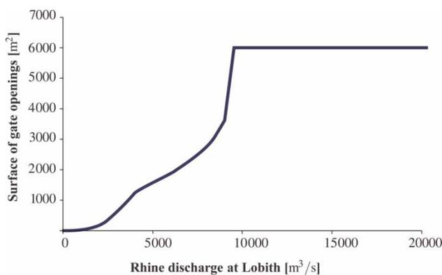
**Figure 6** | The relation that determines the gate openings of the Haringvliet sluices depending on the discharge of the river Rhine at Lobith (van Overloop 2009).
