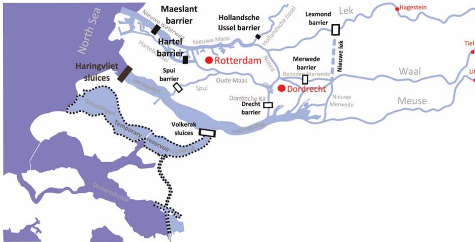
**Figure 3** | A future situation of the Rhine–Meuse delta water system. The Volkerak sluices and the temporary reservoir, as well as the Spui, Drecht, Merwede and Lexmond barriers, provide new control options.
