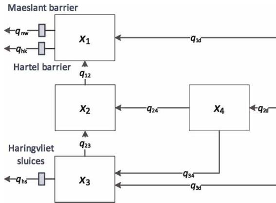
Figure 4 | Structure of the Rhine–Meuse delta model.
