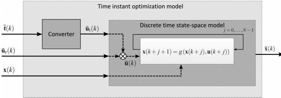
Figure 9 | A possible prediction model structure for TIO-MPC.
