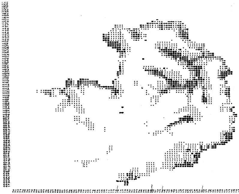
Fig. 7. Synthetic image of Landsat band 5 radiance on July 1, for the Williams Fork Watershed, Colorado, in grey-mapped form. Eight classes ranging from 0 to 320 radiometer counts. Original scale 1:75,000.
