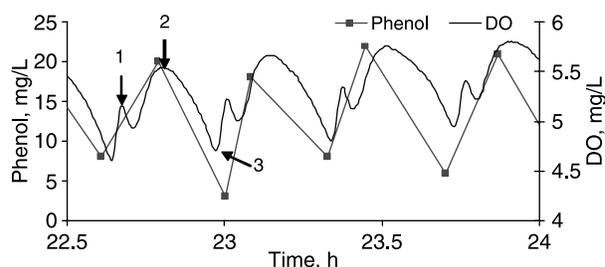
**Figure 5** Detail of degradation kinetic of a mixture of municipal wastewater and 7000 mg/L of phenol using the ED-TOC strategy. The points correspond to the explanation of the points in Figure 2
