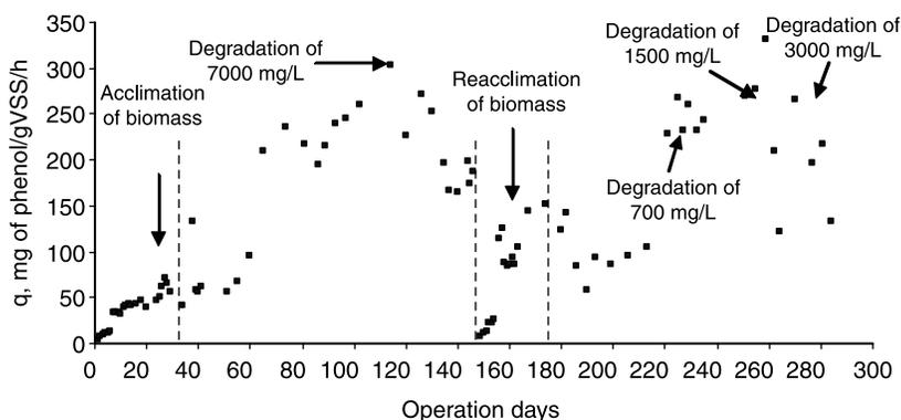
**Figure 3** Specific degradation rate ( $q$ ), during the operation of SBR
