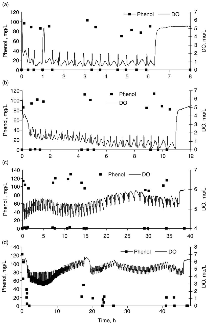
**Figure 4** Degradation kinetic of a mixture of municipal wastewater: (a) 700; (b) 1500; (c) 3000; and (d) 7000 mg/L of phenol using the ED-TOC strategy
