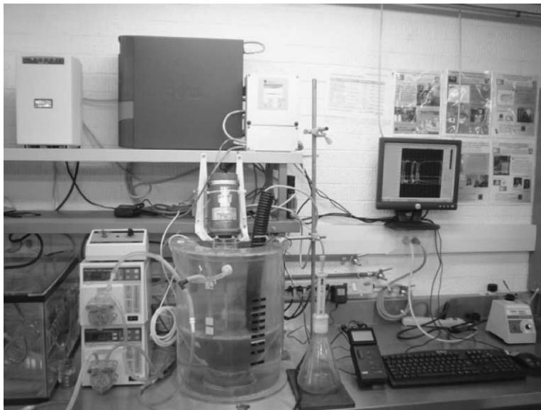
**Figure 1** Experimental assembly showing the reactor set-up
