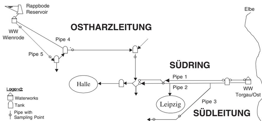
**Figure 1** Scheme of the FWV Elbaue-Ostharz long distance DS
