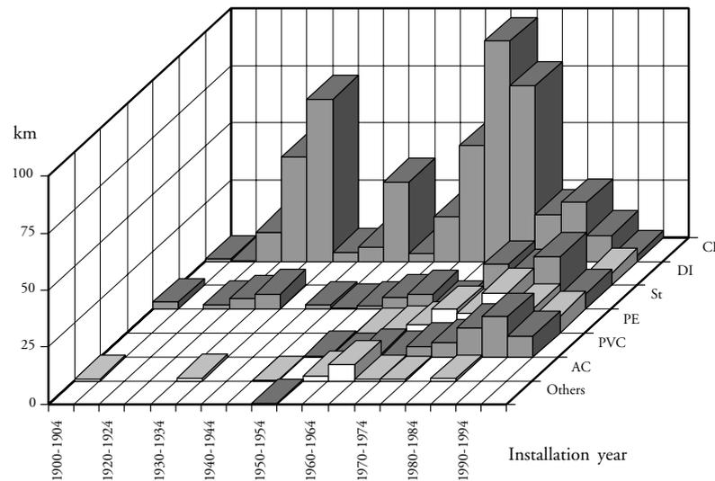
**Fig. 2** Length of water mains in Teplice by period of installation and by material.
