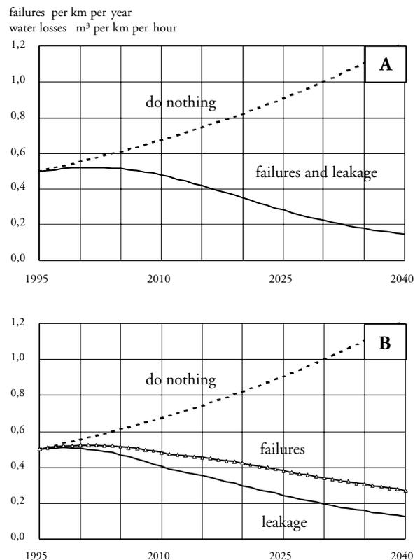
**Fig. 7** Network failure, leakage rate and strategy forecasts.
