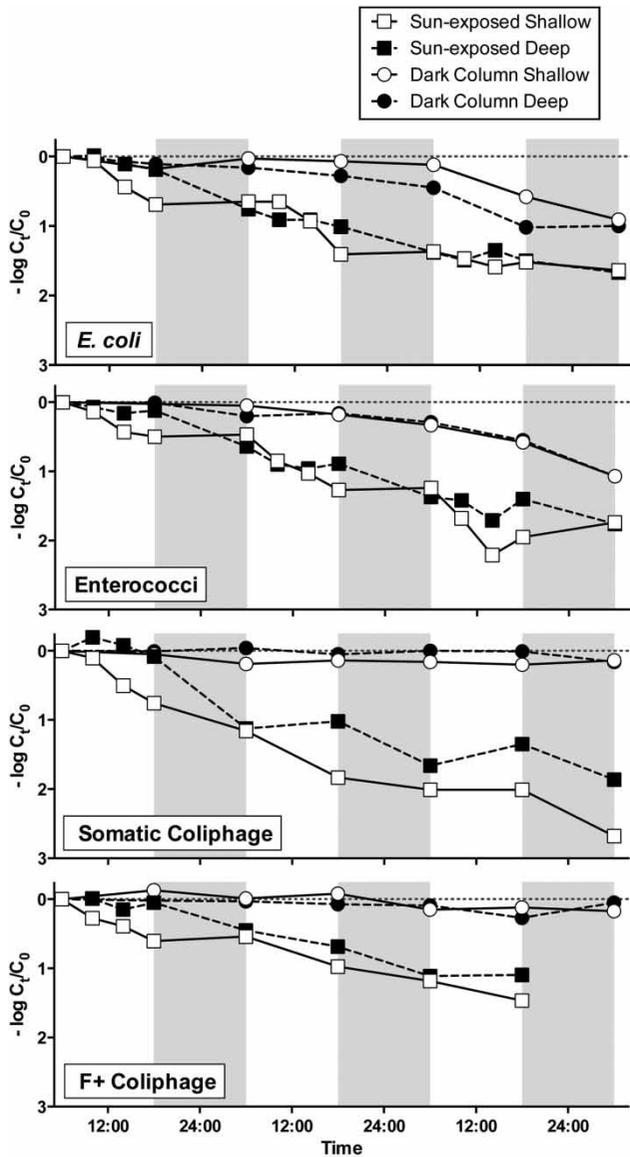
**Figure 3** | Bacteria and coliphage removal measured at each sampling location during Experiment 1. Shaded areas represent night-time.
