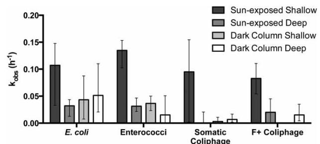
**Figure 4** | Average first-order observed removal rate constants ( $k_{obs}$ ;  $h^{-1}$ ) measured during the day for each microorganism at each sample location during Experiment 1 ( $n = 3$ ).  $k_{obs}$  were calculated between the hours of 6:00 and 18:00. Error bars indicate the range of  $k_{obs}$  values.
