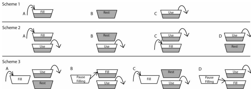
**Figure 7** | Options for treatment pond configuration and operation. For each scheme, A to D illustrate the order of operation.
