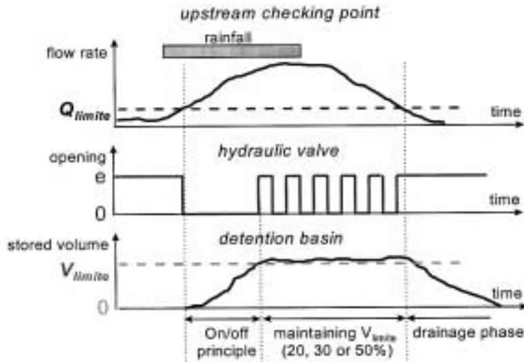
**Figure 4** Principle of the regulations based on the “on/off” operation
