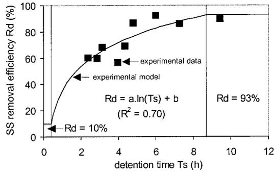
**Figure 6** Experimental model of basin sedimentation efficiency build for the Périnot site
