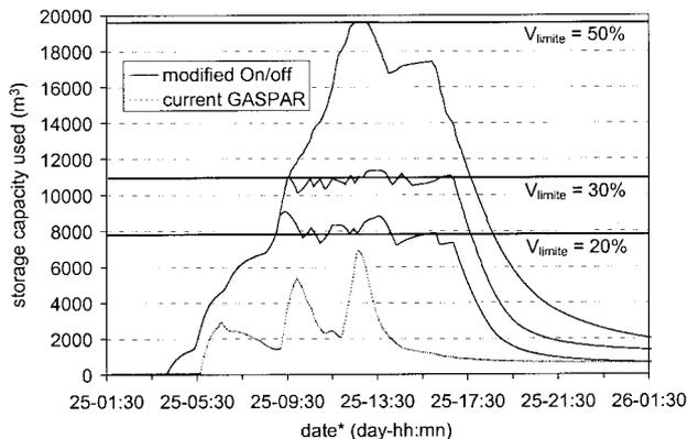
**Figure 5** Distribution of the water volume stored in the Périnot basin (80,000 m<sup>3</sup>) controlled by the current GASPAR regulation and modified “on/off” regulations
