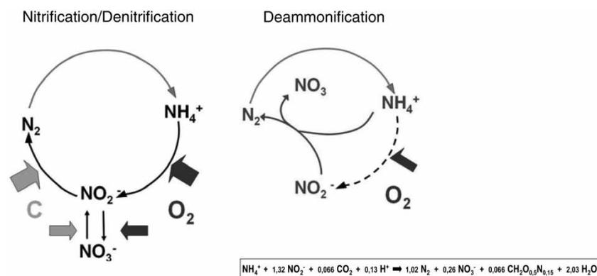
**Figure 2** | Nitrogen elimination process scheme and equation for Anamox process (Strauss et al. 1999).
