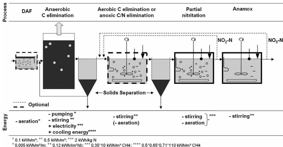
Figure 3 | Coupled nitrogen/carbon removal and energy recovery system.
