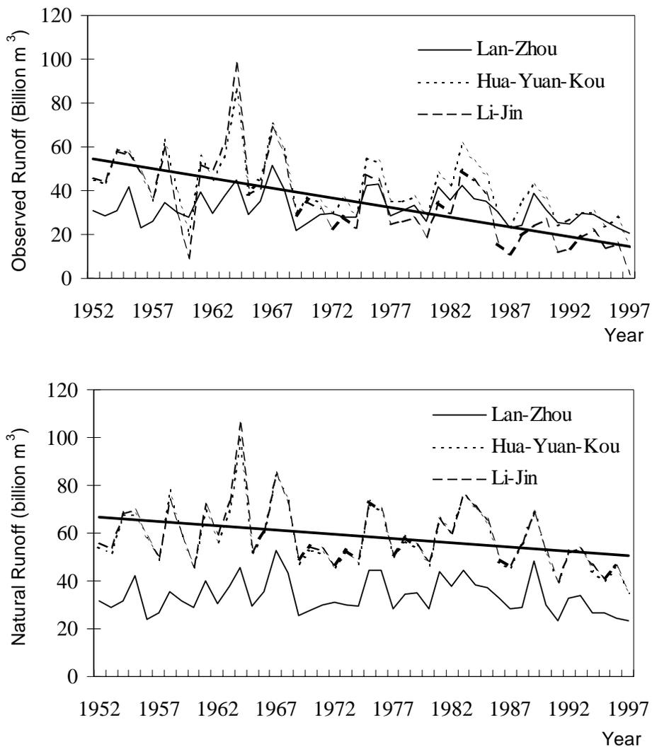
Figure 1 The observed and natural runoff of the Yellow River (1952-1997)
