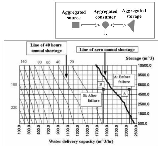
Figure 1 | Shortages analysis—storage versus water delivery capacity.
