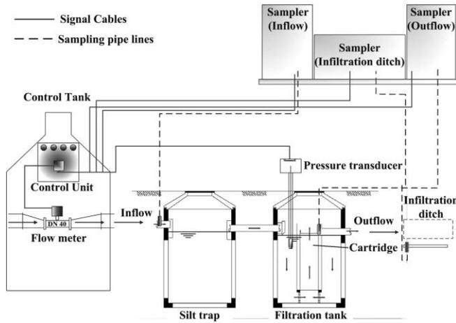
**Figure 1** Technical infiltration system from KME-Mall with monitoring devices
